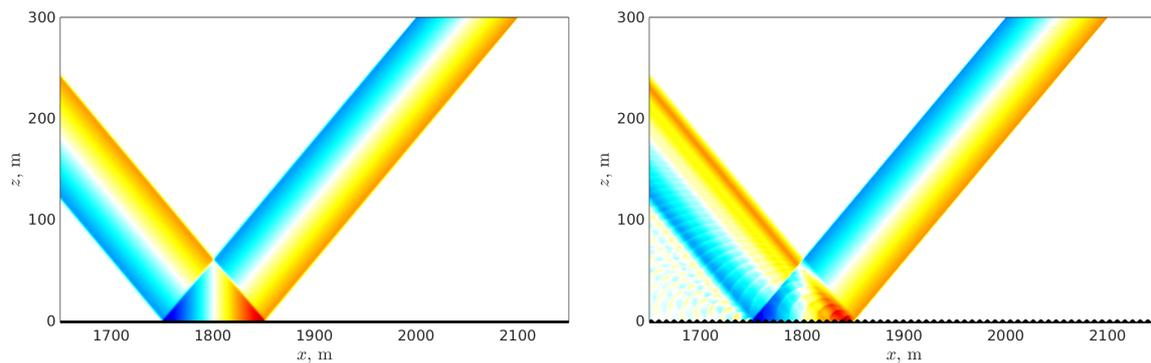
Figure 2: Preliminary numerical simulation of the propagation of a sonic boom in the atmosphere: snapshots of the acoustic pressure above (left) a flat ground and (right) a ground with a sinusoidal profile.
