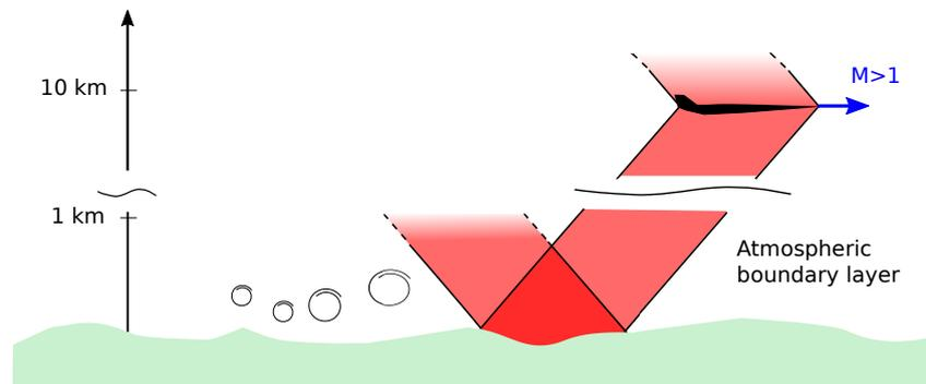
Figure 1: Sonic boom generated by a supersonic aircraft propagating in the atmosphere.
