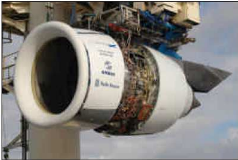
Figure 7. Zero Splice Intake installed on the Rolls-Royce test bed
