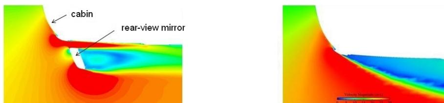
*Figure 1* : Influence of a rear-view mirror on the velocity flow field around a typical cabin of long-haul vehicle (top view) ; with (left) and without (right) rear-view mirror.
