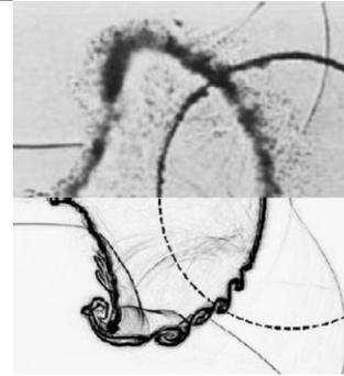
Figure 3: Comparison between numerics (bottom) and experiment (top) of an R22 bubble in air hit by a shock wave (from the right). From Capuano, Bogey & Spelt (2018).
