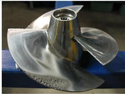
Figure 1: Erosion due to cavitation.
