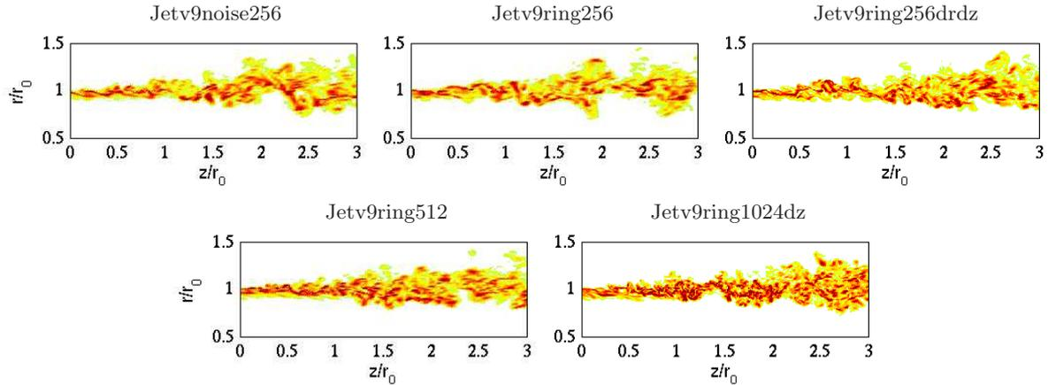
Figure 5. Snapshots in the  $(z, r)$  plane of vorticity norm  $|\omega|$  just downstream of the pipe lip for the different jets. The color scale ranges up to the level of  $25u_j/r_0$ .
