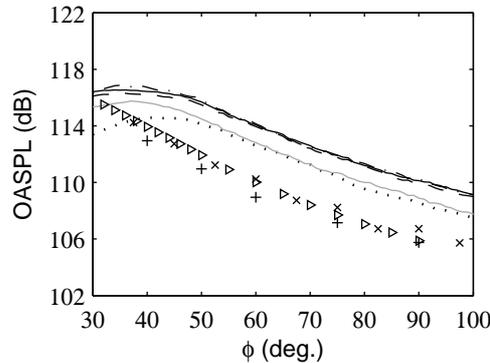
Figure 15. Sound pressure levels obtained at  $60r_0$  from the pipe exit, as functions of the radiation angle relative to the jet direction, for: — Jetv9noise256, - - - Jetv9ring256, - · - · Jetv9ring256drdz, · · · · · Jetv9ring512, ——— Jetv9ring1024dz. Measurements for jets at  $Re_D \geq 5 \times 10^5$ : + Mollo-Christensen *et al.*,<sup>51</sup> × Lush,<sup>52</sup> ▷ Bogey *et al.*<sup>54</sup>
