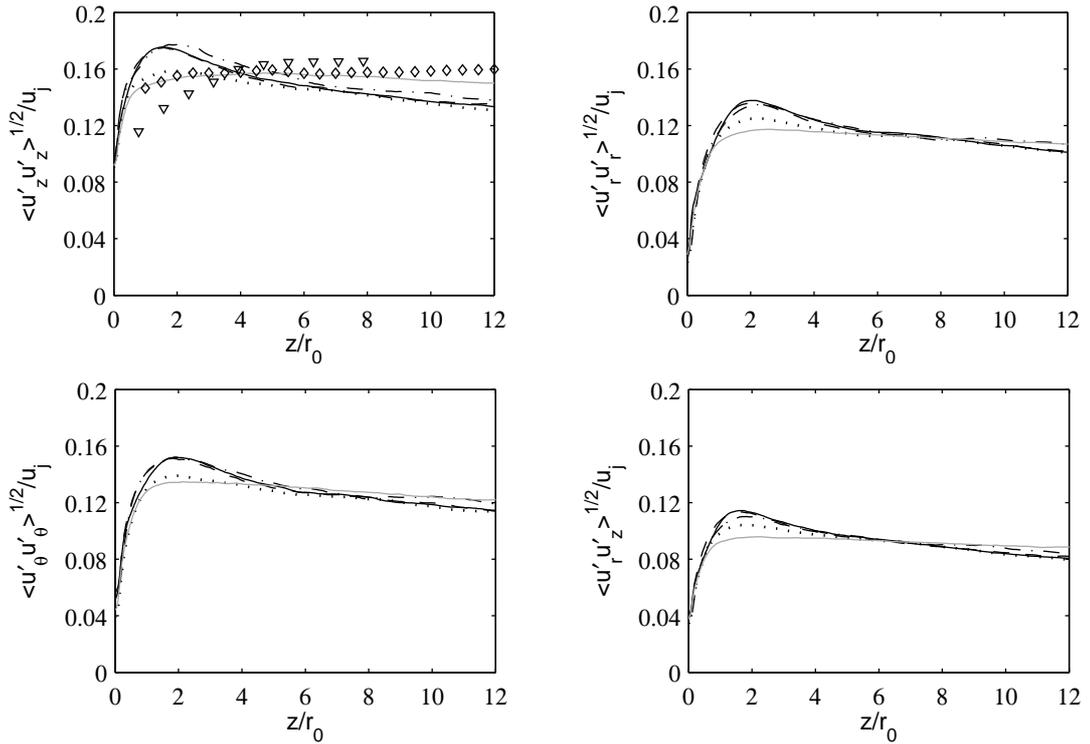
Figure 9. Variations of the peak rms values of fluctuating velocities  $u'_z$ ,  $u'_r$  and  $u'_\theta$ , and of the peak magnitudes of Reynolds shear stress  $\langle u'_r u'_z \rangle$  for: — Jetv9noise256, - - - Jetv9ring256, - · - · Jetv9ring256drdz, ····· Jetv9ring512, ——— Jetv9ring1024dz. Measurements:  $\nabla$  Husain and Hussain<sup>13</sup> for an initially turbulent axisymmetric shear layer,  $\diamond$  Fleury *et al.*<sup>48</sup> for a Mach 0.9 jet at  $Re_D = 7.7 \times 10^5$ .
