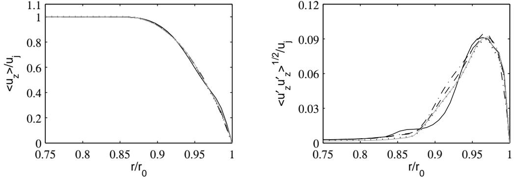
Figure 3. Profiles at  $z = 0$  of mean axial velocity  $\langle u_z \rangle$ , and of the rms values of fluctuating axial velocity  $u'_z$ , for: — Jetv9noise256, - - - Jetv9ring256, - · - · Jetv9ring256drdz, ····· Jetv9ring512, ——— Jetv9ring1024dz.
