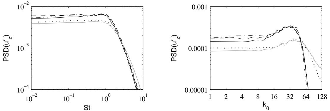
Figure 4. Power spectral densities of axial fluctuating velocity  $u'_z$  as functions of Strouhal number  $St = fD/u_j$  (left), and of azimuthal wave number  $k_\theta$  (right), at  $z = 0.4r_0$  and  $r = r_0$  for: — Jetv9noise256, - - - Jetv9ring256, - · - · Jetv9ring256drdz, ····· Jetv9ring512, ——— Jetv9ring1024dz.
