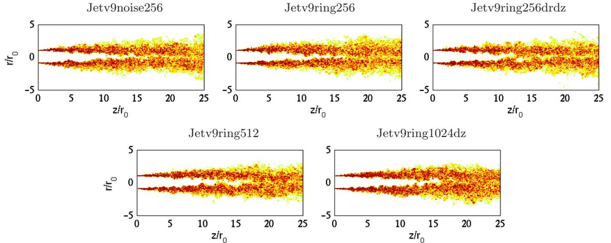
**Figure 10.** Snapshots in the  $(z, r)$  plane of vorticity norm  $|\omega|$  for the jet flow fields up to  $z = 25r_0$ . The color scale ranges up to the level of  $5u_j/r_0$ .
