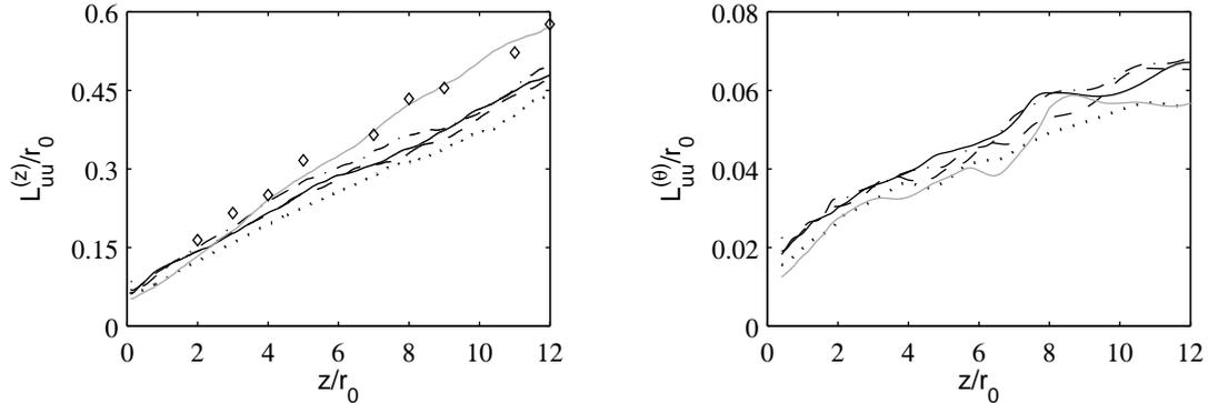
**Figure 6.** Variations along the lip line of the axial and azimuthal integral length scales  $L_{uu}^{(z)}$  and  $L_{uu}^{(\theta)}$  calculated from velocity  $u'_z$  at  $r = r_0$  for: — Jetv9noise256, - - - Jetv9ring256, - · - · Jetv9ring256drdz, ····· Jetv9ring512, ——— Jetv9ring1024dz. Measurements:  $\diamond$  Fleury *et al.*<sup>48</sup> for a Mach 0.9 jet at  $Re_D = 7.7 \times 10^5$ .
