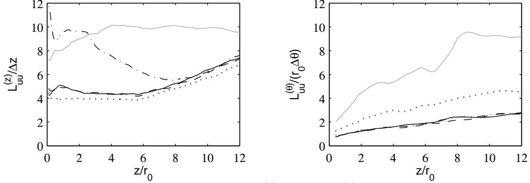
Figure 7. Variations along the lip line of the ratios  $L_{uu}^{(z)}/\Delta z$  and  $L_{uu}^{(\theta)}/(r_0\Delta\theta)$  between integral length scales calculated from velocity  $u'_z$ , and mesh spacings, for:  $\text{—}$  *Jetv9noise256*,  $\text{-- --}$  *Jetv9ring256*,  $\text{- \cdot - \cdot}$  *Jetv9ring256drdz*,  $\cdots$  *Jetv9ring512*,  $\text{— — — —}$  *Jetv9ring1024dz*.
