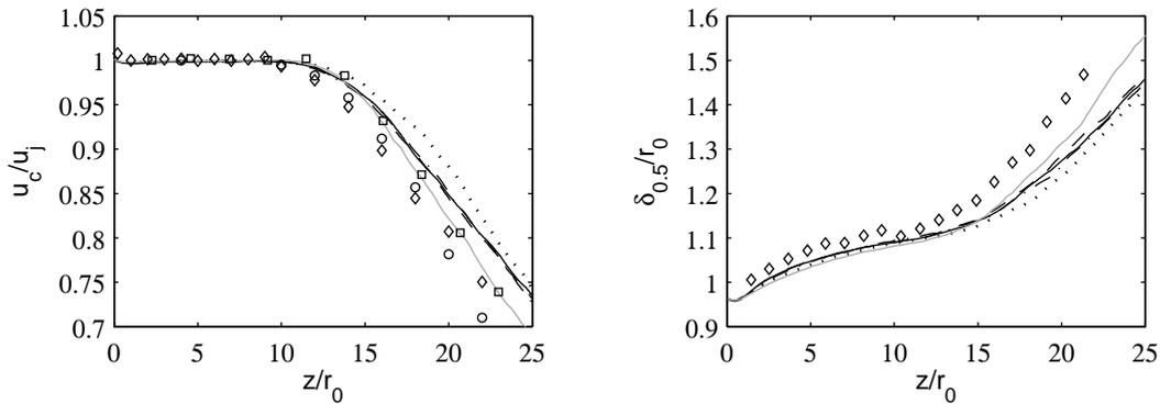
Figure 11. Variations of centerline mean axial velocity  $u_c$  and of jet half-width  $\delta_{0.5}$  for: — Jetv9noise256, - - - Jetv9ring256, - · - · Jetv9ring256drdz, ····· Jetv9ring512, ——— Jetv9ring1024dz. Measurements for Mach 0.9 jets at  $Re_D \geq 5 \times 10^5$ :  $\circ$  Lau *et al.*,<sup>49</sup>  $\square$  Arakeri *et al.*,<sup>17</sup>  $\diamond$  Fleury *et al.*<sup>48</sup>
