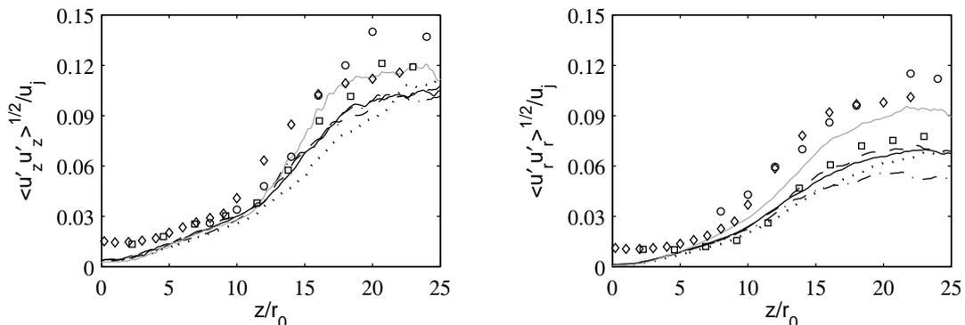
Figure 12. Variations along jet centerline at  $r = 0$  of the rms values of fluctuating velocities  $u'_z$  and  $u'_r$  for: — Jetv9noise256, - - - Jetv9ring256, - · - · Jetv9ring256drdz, ····· Jetv9ring512, ——— Jetv9ring1024dz. Measurements for Mach 0.9 jets at  $Re_D \geq 5 \times 10^5$ :  $\circ$  Lau *et al.*,<sup>49</sup>  $\square$  Arakeri *et al.*,<sup>17</sup>  $\diamond$  Fleury *et al.*<sup>48</sup>
