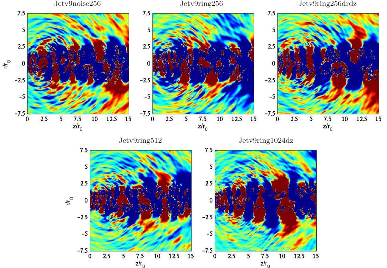
Figure 13. Snapshots in the  $(z, r)$  plane of fluctuating pressure  $p - p_{amb}$  obtained by LES for the different jets. The color scale ranges for levels from -100 Pa to 100 Pa.
