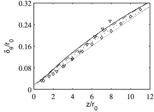
Figure 8. Variations of shear-layer momentum thickness  $\delta_\theta$  for: — Jetv9noise256, - - - Jetv9ring256, - · - · Jetv9ring256drdz, ····· Jetv9ring512, ——— Jetv9ring1024dz. Measurements:  $\nabla$  Husain and Hussain<sup>13</sup> for an initially turbulent axisymmetric shear layer,  $\diamond$  Fleury *et al.*<sup>48</sup> for a Mach 0.9 jet at  $Re_D = 7.7 \times 10^5$ .
