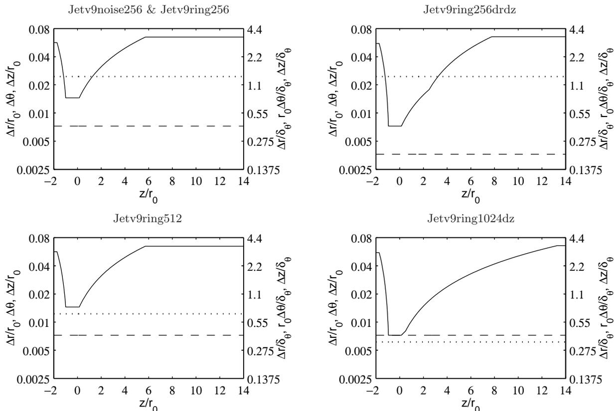
Figure 2. Representation, in logarithmic scales, of the mesh spacings in the axial, radial and azimuthal directions at  $r = r_0$ , in the different simulations: —  $\Delta z$ , - - -  $\Delta r$ , .....  $r_0 \Delta \theta$ . They are normalized by the jet radius  $r_0$  (left  $y$ -axis) or by the exit boundary-layer momentum thickness  $\delta_\theta$  (right  $y$ -axis).
