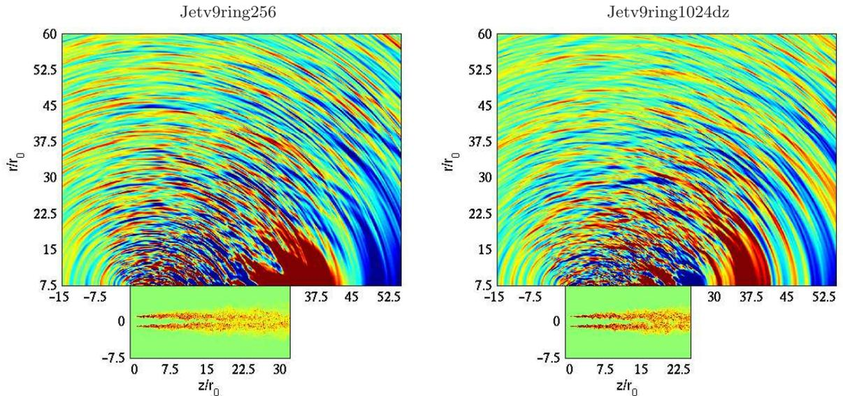
Figure 14. Snapshots in the  $(z, r)$  plane of the pressure field obtained from the acoustical simulations for Jetv9ring256 and Jetv9ring1024dz. The color scale ranges for levels from -16 Pa to 16 Pa.
