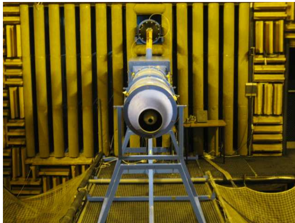
Figure 1. Photograph of the free jet flight simulating facility built in an anechoic environment.
