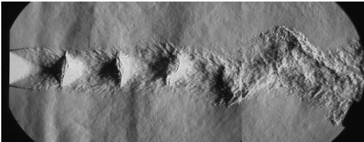
Figure 17. Collage from three spark Schlieren pictures of the supersonic jet plume. M_j = 1.50 , M_f = 0.39 . Exposure time is 6.7 \mu s .
