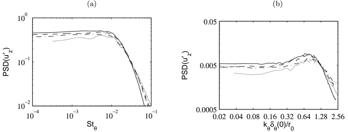
**Figure 2.** Power spectral densities (PSD) normalized by  $u_j$  of fluctuating velocity  $u'_z$  at  $r = r_0$  and  $z = 22\delta_\theta(0)$ , as functions (a) of  $St_\theta = f\delta_\theta(0)/u_j$  and (b) of  $k_\theta\delta_\theta(0)/r_0$ , for ——— Jetring512, - - - Jetring1024dz, - · - · - Jetring1024drdz, — — — Jetring1024drdz2 $\delta_\theta$ .
