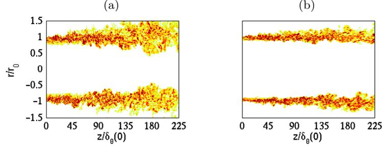
Figure 4. Snapshots in the  $(z, r)$  plane of vorticity norm from (a) `Jetring1024drdz2δθ` and (b) `Jetring1024drdz`. The  $z$ -axis is normalized by  $\delta_\theta(0)$ . The colour scales range up to the level of (a)  $11.25u_j/r_0$  and (b)  $15u_j/r_0$ .
