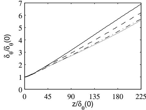
Figure 5. Variations of shear-layer momentum thickness  $\delta_\theta/\delta_\theta(0)$ , as functions of  $z/\delta_\theta(0)$ , for ——— `Jetring512`, - - - `Jetring1024dz`, - · - · `Jetring1024drdz`, ——— `Jetring1024drdz2δθ`.
