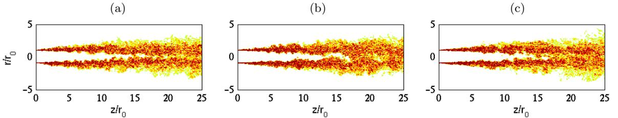
Figure 8. Snapshots in the  $(z, r)$  plane of vorticity norm in the full jets up to  $z = 25r_0$ : (a) *Jetring512*, (b) *Jetring1024dz*, (c) *Jetring1024drdz*. The colour scales range up to the level of  $5u_j/r_0$ .
