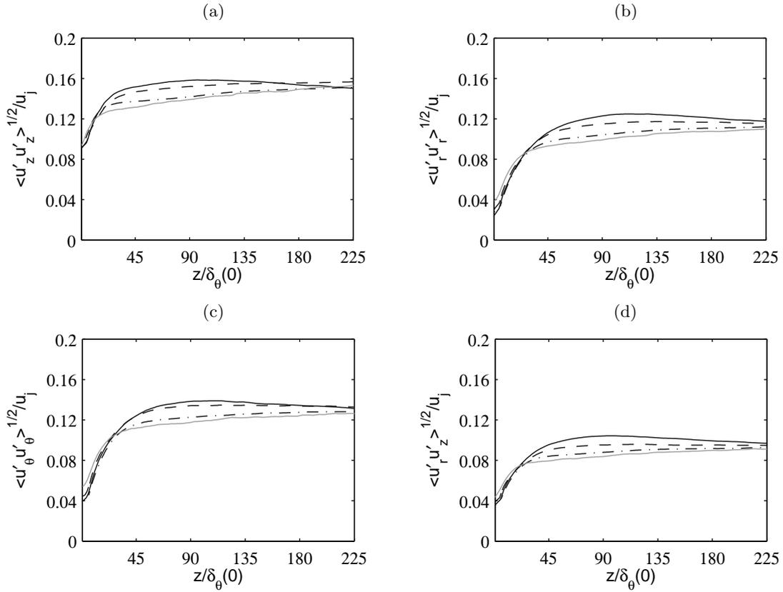
Figure 6. Variations of the peak rms values of velocities (a)  $u'_z$ , (b)  $u'_r$  and (c)  $u'_\theta$ , and (d) of the peak magnitudes of Reynolds shear stress  $\langle u'_r u'_z \rangle$ , as functions of  $z/\delta_\theta(0)$ , for  $\text{---}$  Jetring512,  $\text{- - -}$  Jetring1024dz,  $\text{- \cdot - \cdot}$  Jetring1024drdz,  $\text{---}$  Jetring1024drdz2 $\delta_\theta$ .
