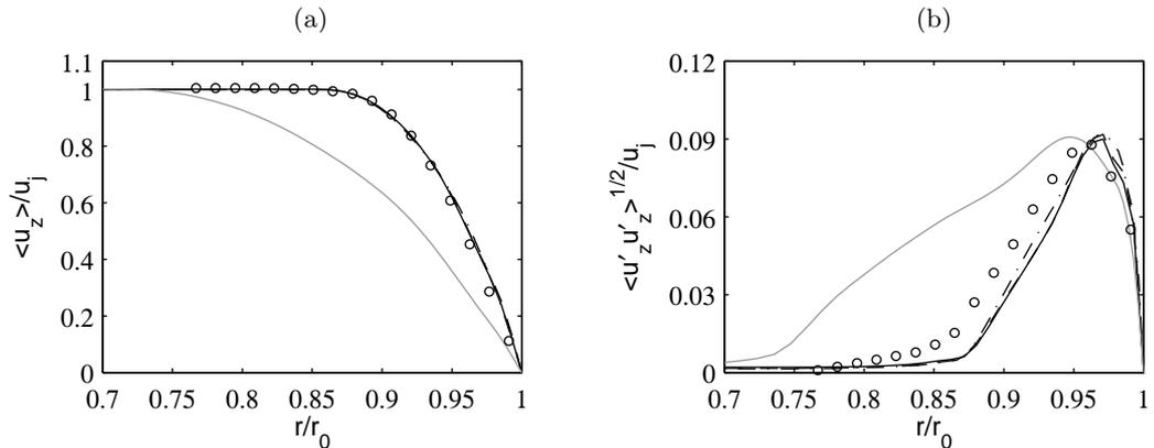
Figure 1. Profiles at  $z = 0$  (a) of mean axial velocity  $\langle u_z \rangle$ , and (b) of the rms values of fluctuating axial velocity  $u'_z$  for — Jetring512, - - - Jetring1024dz, - · - · Jetring1024drdz, — Jetring1024drdz2 $\delta_\theta$ . Measurements for a Mach 0.18, tripped jet at  $Re_D = 10^5$ :  $\circ$  Zaman.<sup>11,12</sup>
