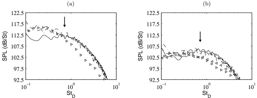
Figure 11. Sound pressure levels (SPL) at  $60r_0$  from the jet exit, as functions of  $St_D = fD/u_j$ , at the angles of (a)  $40^\circ$  and (b)  $90^\circ$ , for ——— Jetring512, - - - Jetring1024dz, - · - · Jetring1024drdz. The arrows indicate the frequency determined using  $St_\theta = f\delta_\theta(0)/u_j = 0.0065$ . Measurements for jets at  $Re_D \geq 7.8 \times 10^5$ :  $\triangleleft$  Tanna,<sup>36</sup>  $\triangleright$  Bogey *et al.*<sup>37</sup>
