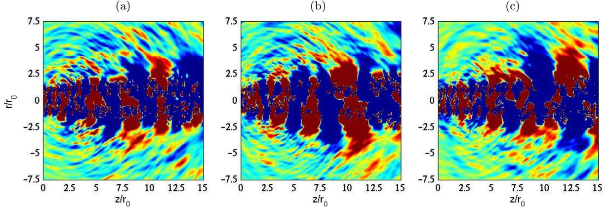
Figure 10. Snapshots in the  $(z, r)$  plane of fluctuating pressure: (a) Jetring512, (b) Jetring1024dz, (c) Jetring1024drdz. The colour scale ranges from levels of -100 Pa to 100 Pa.
