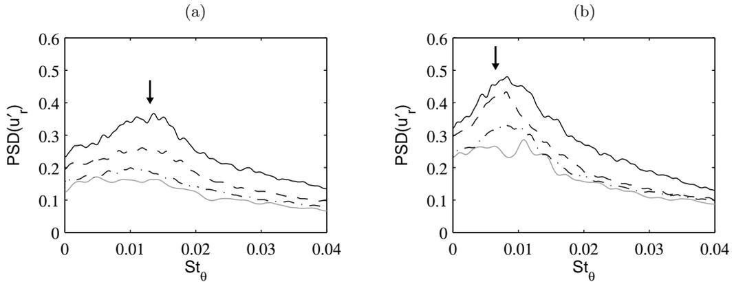
Figure 7. Power spectral densities (PSD) normalized by  $u_j$  of radial velocity  $u'_r$ , (a) at  $r = r_0$  and  $z = 83\delta_\theta(0)$  and (b) at  $r = r_0$  and  $z = 166\delta_\theta(0)$ , as functions of  $St_\theta = f\delta_\theta(0)/u_j$ , for  $\text{---}$  Jetring512,  $\text{- - -}$  Jetring1024dz,  $\text{- \cdot - \cdot}$  Jetring1024drdz,  $\text{---}$  Jetring1024drdz2 $\delta_\theta$ . The arrows indicate (a)  $St_\theta = 0.013$  and (b)  $St_\theta = 0.0065$ .
