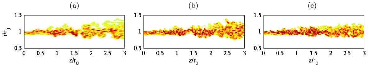
**Figure 3.** Snapshots in the  $(z, r)$  plane of vorticity norm in the shear layers just downstream of the pipe lip: (a) Jetring512, (b) Jetring1024dz, (c) Jetring1024drdz. The colour scales range up to the level of  $25u_j/r_0$ .
