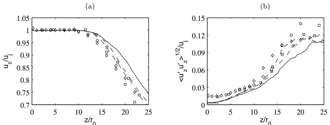
Figure 9. Variations (a) of centerline mean axial velocity  $u_c$  and (b) of centerline rms values of velocity  $u'_z$ , for — *Jetring512*, - - - *Jetring1024dz*, - · - · *Jetring1024drdz*. Measurements for Mach 0.9 jets at  $Re_D \geq 5 \times 10^5$ :  $\circ$  Lau *et al.*,<sup>33</sup>  $\square$  Arakeri *et al.*,<sup>34</sup>  $\diamond$  Fleury *et al.*<sup>35</sup>
