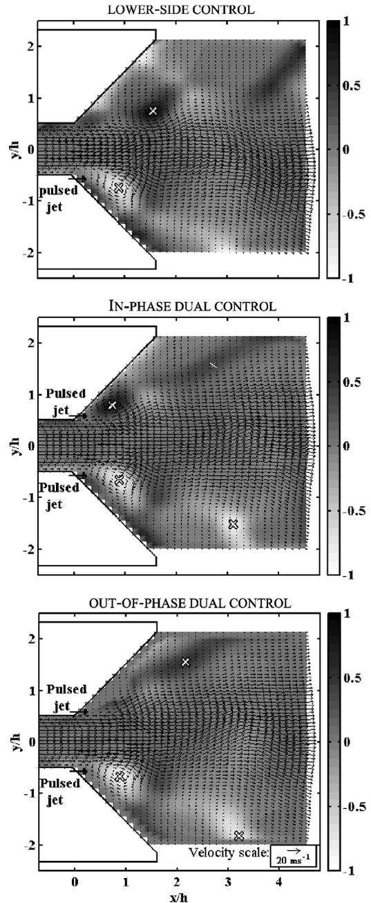
Fig. 5 Phase-average velocity fields ( $\rightarrow$ ) and corresponding maps of phase-average eddy-center criterion (gray level and crosses) at the end of the blowing phase of the lower actuator.
