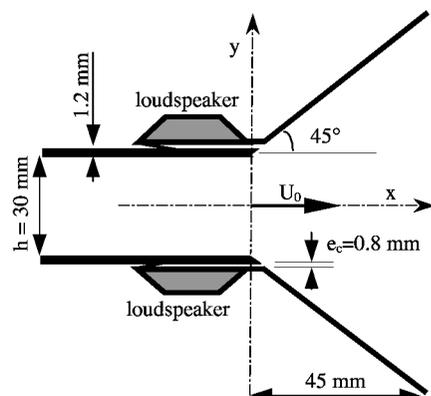
Fig. 1 Schematic of the experiment and axis definitions.
