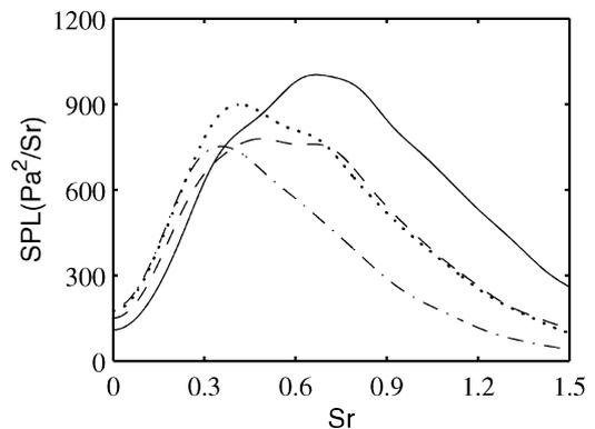
**Fig. 4** Sound-pressure spectra as a function of Strouhal number  $Sr = fD/u_j$ , in linear scales, obtained in the sideline direction at  $x = 11r_0$  and  $r = 15r_0$  from —, LESsf; . . . ., LESdsm; ---, LESre1; and - - - -, LESre2 simulations.
