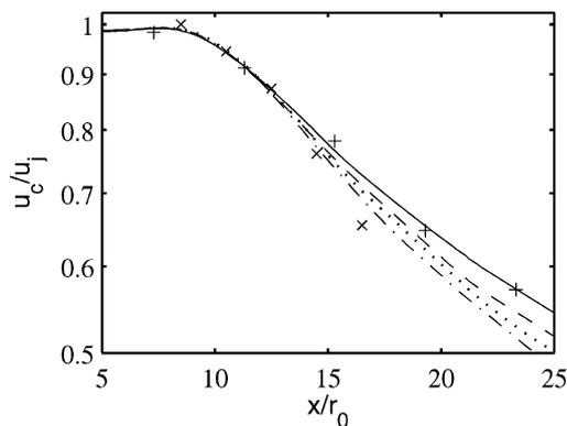
**Fig. 2** Profiles of the mean centerline velocity  $u_c/u_j$  in —, LESsf; . . . ., LESdsm; ---, LESre1; and - - - -, LESre2 simulations. Measurements: x, Stromberg et al.<sup>13</sup> ( $M = 0.9$ ,  $Re_D = 3.6 \times 10^3$ ) and +, Lau et al.<sup>14</sup> ( $M = 0.9$ ,  $Re_D = 10^6$ ). The LESdsm, LESre1, LESre2, and experimental profiles are shifted in the axial direction with respect to the LESsf profile to yield identical core lengths.
