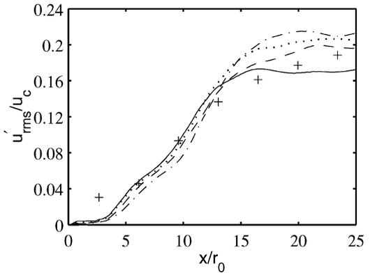
**Fig. 3** Centerline profiles of the turbulence intensity  $u'_{rms}/u_c$  in —, LESsf; . . . ., LESdsm; ---, LESre1; and - - - -, LESre2 simulations. Measurements: +, Arakeri et al.<sup>15</sup> ( $M = 0.9$ ,  $Re_D = 5 \times 10^5$ ), shifted in the axial direction for the comparison.
