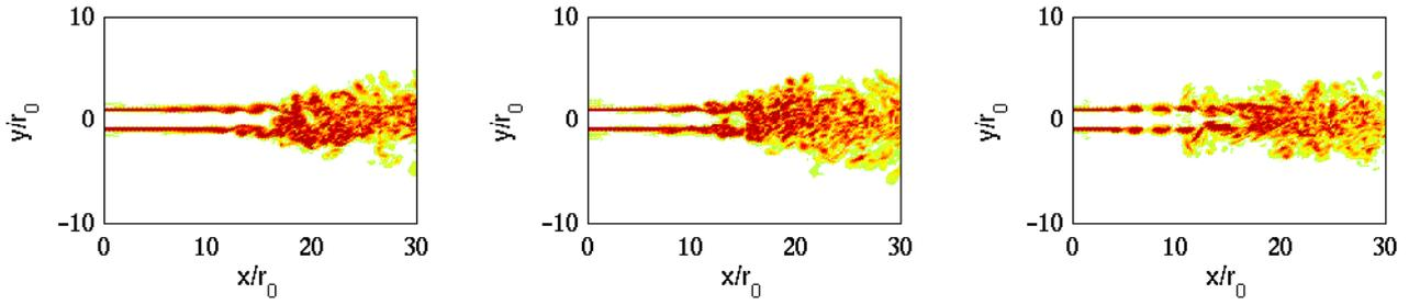
FIG. 2 – Snapshots of vorticity norm normalized by the jet diameter and inflow velocity,  $|\omega|D/u_j$ , in the plane  $z = 0$ , for : jetRe3600, jetRe3600thin and jetRe3600mode, from left to right. The color scale ranges for levels from 0.6 to 3.
