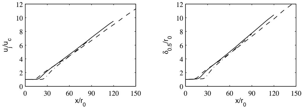
FIG. 3 – Variations of the inverse of centerline mean axial velocity  $u_j/u_c$  (left) and of the jet half-width  $\delta_{0.5}/r_0$  (right), for :  $\cdots$  jetRe1800,  $\text{—}$  jetRe3600, and  $\text{-- --}$  jetRe11000.
