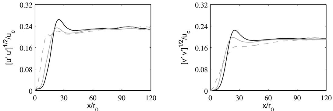
FIG. 6 – Variations along the jet centerline of axial and radial turbulence intensities  $[u'u']^{1/2}/u_c$  (left) and  $[v'v']^{1/2}/u_c$  (right), for :  $\text{—}$  jetRe3600,  $\text{-- --}$  jetRe3600thin, and  $\cdots$  jetRe3600mode.
