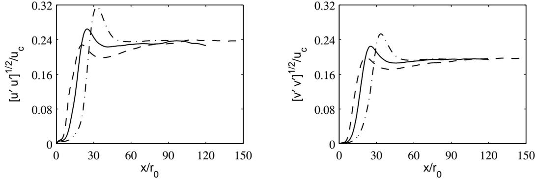
FIG. 5 – Variations along the jet centerline of axial and radial turbulence intensities  $[u'u']^{1/2}/u_c$  (left) and  $[v'v']^{1/2}/u_c$  (right), for :  $\cdots$  jetRe1800,  $\text{—}$  jetRe3600, and  $\text{-- --}$  jetRe11000.
