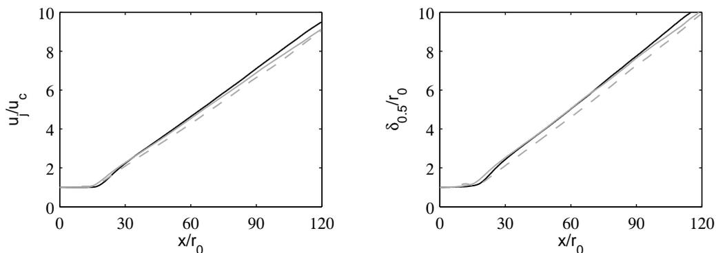
FIG. 4 – Variations of the inverse of centerline mean axial velocity  $u_j/u_c$  (left) and of the jet half-width  $\delta_{0.5}/r_0$  (right), for :  $\text{—}$  jetRe3600,  $\text{-- --}$  jetRe3600thin, and  $\cdots$  jetRe3600mode.
