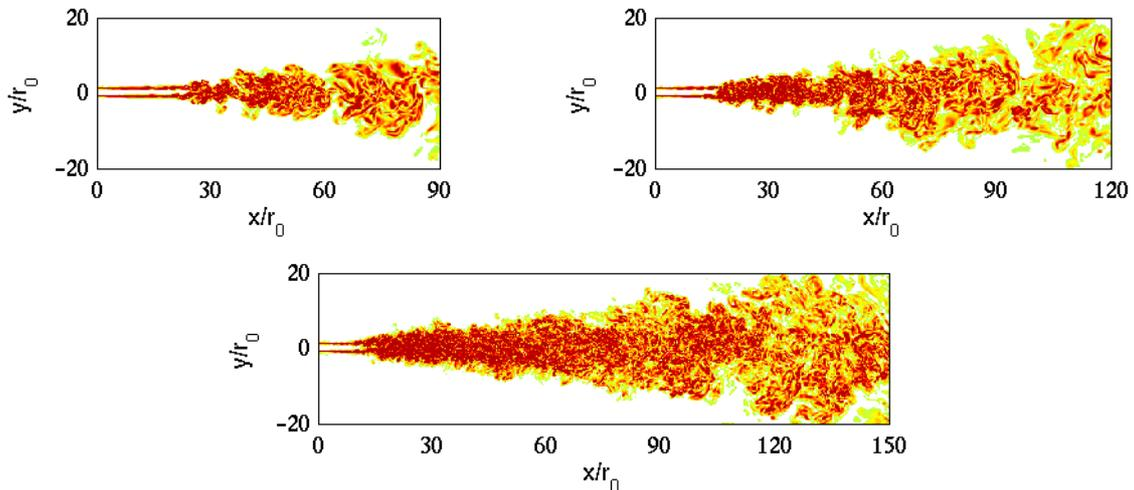
FIG. 1 – Snapshots of vorticity norm normalized by the jet diameter and the centerline mean axial velocity,  $|\omega|D/u_c$ , in the plane  $z = 0$ , for : jetRe1800 (top left), jetRe3600 (top right) and jetRe11000 (bottom). The color scale ranges for levels from 0.4 to 2.
