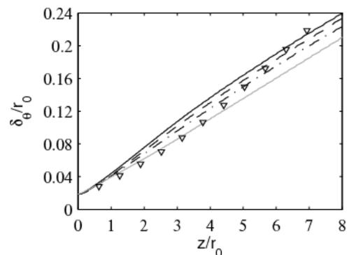
Fig.2. Shear-layer momentum thickness at  $r=r_0$  for: Jetv9ring256 (black solid line), Jetv9ring256fine (black dashed line), Jetv9ring512 (black mixed line), Jetv9ring1024 (grey solid line). Measurements for an initially turbulent shear layer: [2].
