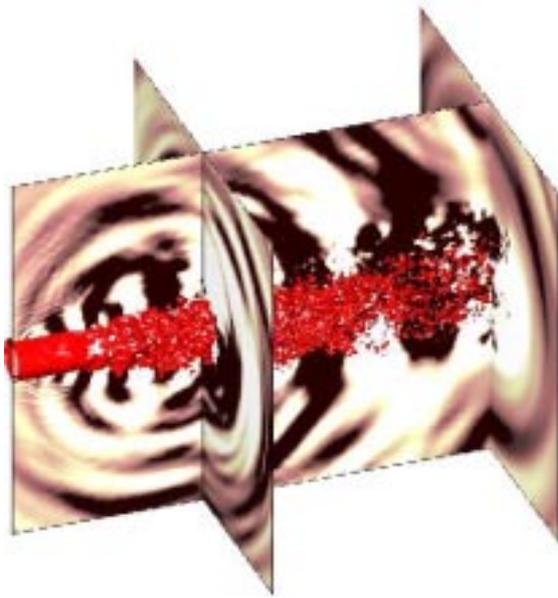
Figure 4 : LES simulation of a high Mach number, high Reynolds number subsonic jet. Visualisation of the flow region (norm of the vorticity vector) and of the acoustic region (pressure field).
