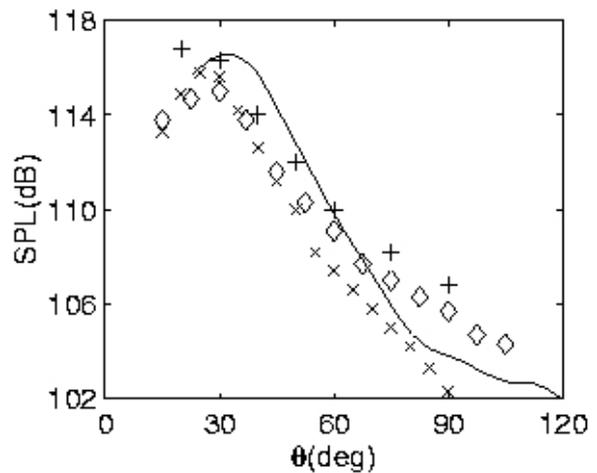
Figure 3 : Directivity of noise emission of a jet at Mach 0.9 (- numerical simulation,  $Re=65000$ ; x experimental data,  $Re=3600$ , + and diamonds,  $Re=5 \cdot 10^5$ ). see ref. [8] for details
