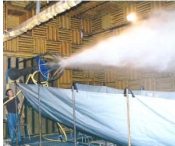
Figure 1 : Injection of water in a supersonic air-jet to reduce the generated noise (Mach=1.3)
