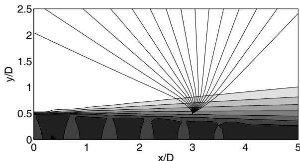
Figure 3: Ray-tracing algorithm for a source located in a shocked jet,  $M_j = 1.35$ . The velocity field is shown, the color scale ranges for levels from 0 to 400 m/s, from white to gray. The ray paths are shown in straight lines.
