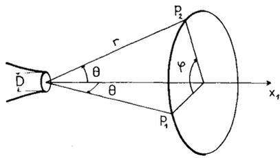
Fig. 1 Geometry for two microphone correlations.
