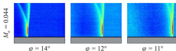
Fig. 3. (Color online) Three consecutive schlieren images from the high-speed camera obtained for the same position of the spark source ( $M_a = 0.044$  for the first frame).
