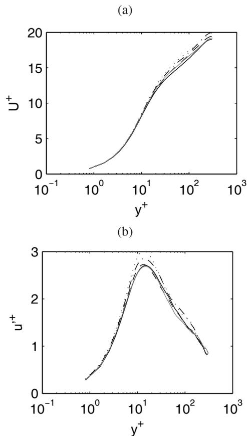
Figure 2: Grid convergence in the  $z$  direction: (a) mean, and (b) rms streamwise velocities.  $\cdots\cdots$  Gdz1 ( $\Delta z^+ = 15$ ),  $-\cdot-\cdot-$  Gdz2 ( $\Delta z^+ = 12.5$ ),  $---$  Gdz3 ( $\Delta z^+ = 10$ ),  $—$  Gdz4 ( $\Delta z^+ = 7.5$ ),  $—$  Gdz5 ( $\Delta z^+ = 5$ ).
