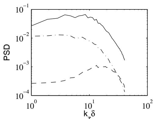
Figure 5: Power spectral densities of velocity fluctuations, at a distance to the wall  $y^+ = 13$ , as a function of the spanwise wavenumber scaled by the boundary layer thickness  $\delta = 0.9h$ : —  $\Phi_{uu}$ , - - -  $\Phi_{vv}$ , - · - ·  $\Phi_{ww}$ .
