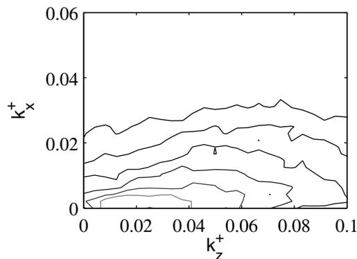
Figure 7: Power spectral density of the streamwise velocity fluctuations  $\Phi_{uu}$ , at a distance to the wall  $y^+ = 13$ , as a function of the streamwise ( $k_x$ ) and spanwise ( $k_z$ ) wavenumbers, given in wall units. Two consecutive isolines represent a magnitude ratio of 2.
