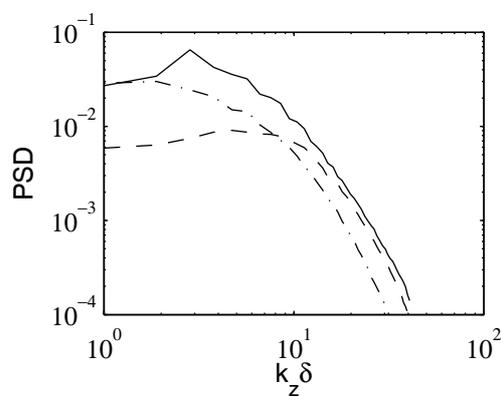
Figure 6: Power spectral densities of velocity fluctuations, at a distance to the wall  $y = 0.3\delta$ , as a function of the spanwise wavenumber scaled by the boundary layer thickness  $\delta = 0.9h$ : —  $\Phi_{uu}$ , - - -  $\Phi_{vv}$ , - · - ·  $\Phi_{ww}$ .
