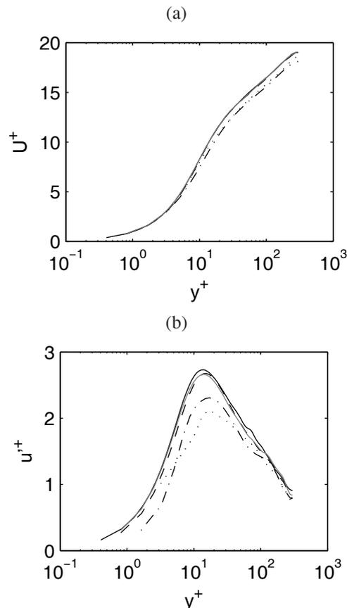
Figure 1: Grid convergence in the y direction: (a) mean, and (b) rms streamwise velocities.  $\cdots\cdots$  Gdy1 ( $\Delta y_w^+ = 3.7$ ),  $-\cdot-\cdot-$  Gdy2 ( $\Delta y_w^+ = 1.9$ ),  $- - -$  Gdy3 ( $\Delta y_w^+ = 0.95$ ),  $—$  Gdy4 ( $\Delta y_w^+ = 0.47$ ),  $—$  Gdy3 ( $\Delta y_w^+ = 0.95$ ) using the semi-implicit time integration scheme (SIRK)
