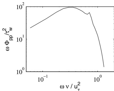
Figure 4: Premultiplied power spectral density of the fluctuating wall pressure scaled by the wall shear stress, as a function of the angular frequency, scaled by the viscous time scale
