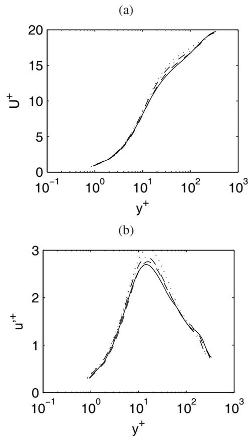
Figure 3: Grid convergence in the  $x$  direction: (a) mean, and (b) rms streamwise velocities.  $\cdots\cdots$  Gdx1 ( $\Delta x^+ = 45$ ),  $-\cdot-\cdot-$  Gdx2 ( $\Delta x^+ = 35$ ),  $---$  Gdx3 ( $\Delta x^+ = 30$ ),  $—$  Gdx4 ( $\Delta x^+ = 15$ ).
