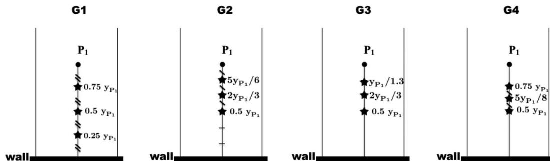
Fig. 9 Representation of the ghost cell positions ( $\star$ ) in the wall-normal direction for LESs G1, G2, G3, and G4.
