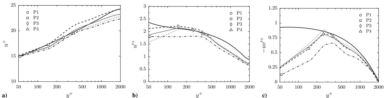
**Fig. 8** Representations of a) mean streamwise velocities, b) rms streamwise velocities, and c) Reynolds shear stresses: LESs using  $P_1$  (dashed-dotted lines),  $P_2$  (dashed lines),  $P_3$  (grey, solid lines) and  $P_4$  (dotted lines); DNS of [32] (black, solid lines).
