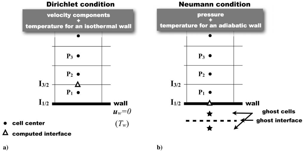
Fig. 6 Spatial discretization close to the wall for the spatial scheme [11] in the case of a wall-modeled LES: a) Dirichlet condition, and b) Neumann condition at the wall.
