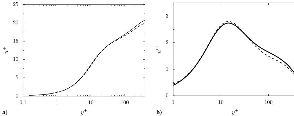
**Fig. A1 Representations of a) mean and b) rms streamwise velocity profiles: LESs using mesh M1 (dashed–dotted lines), M2 (dotted lines), M3 (dashed lines); and DNS of [24] (solid lines).**
