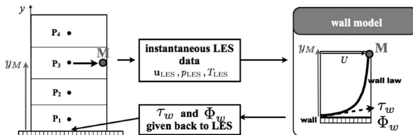
Fig. 5 Wall model application. The values of  $\tau_w$  and  $\Phi_w$  are computed by the model using instantaneous LES data at matching point M.
