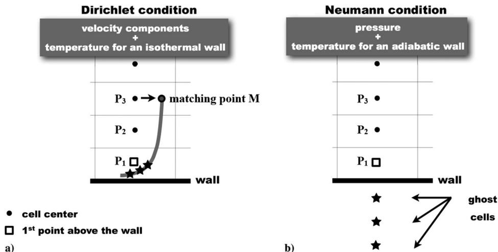
Fig. 7 Spatial discretization close to the wall for the selective filter [13] in the case of a wall-modeled LES: a) Dirichlet condition, and b) Neumann condition at the wall.
