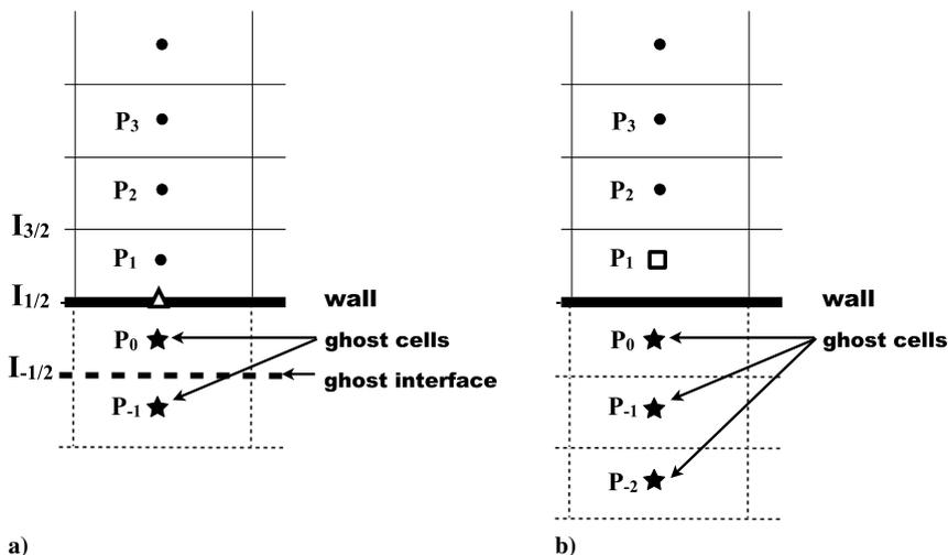
Fig. 3 Spatial discretization for a wall-resolved LES: a) for the spatial scheme [11], and b) for the selective filter [13].
