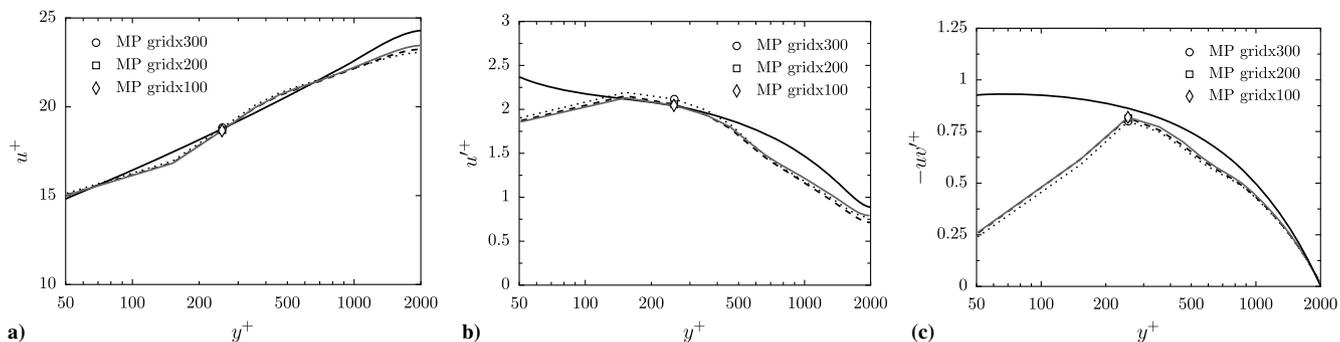
**Fig. 13** Representations of a) mean streamwise velocities, b) rms streamwise velocities, and c) Reynolds shear stresses: LESs using gridx300 (dotted lines), gridx200 (dashed lines), and gridx100 (grey, solid lines); DNS of [32] (black, solid lines).
