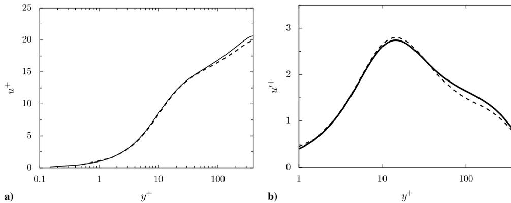
Fig. 4 Streamwise velocity profiles in the channel: a) mean, and b) rms. Dashed lines denote LES, and solid lines denote DNS of [24].
