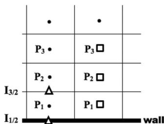
Fig. 2 Representation of interfaces (triangles ( $\Delta$ )) and points (squares ( $\square$ )) for which the spatial scheme and selective filter cannot be applied.
