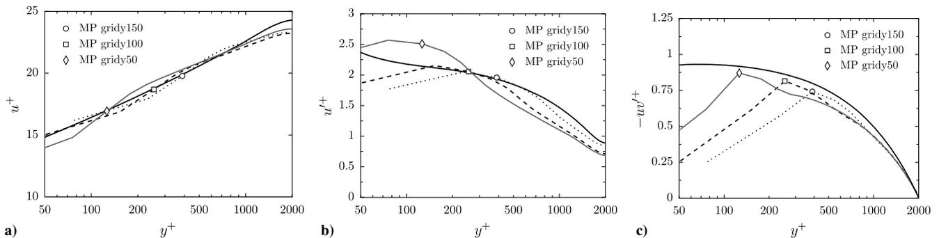
**Fig. 11** Representations of a) mean streamwise velocities, b) rms streamwise velocities, and c) Reynolds shear stresses: LESs using gridy150 (dotted lines), gridy100 (dashed lines), and gridy50 (grey, solid lines); DNS of [32] (black, solid lines).
