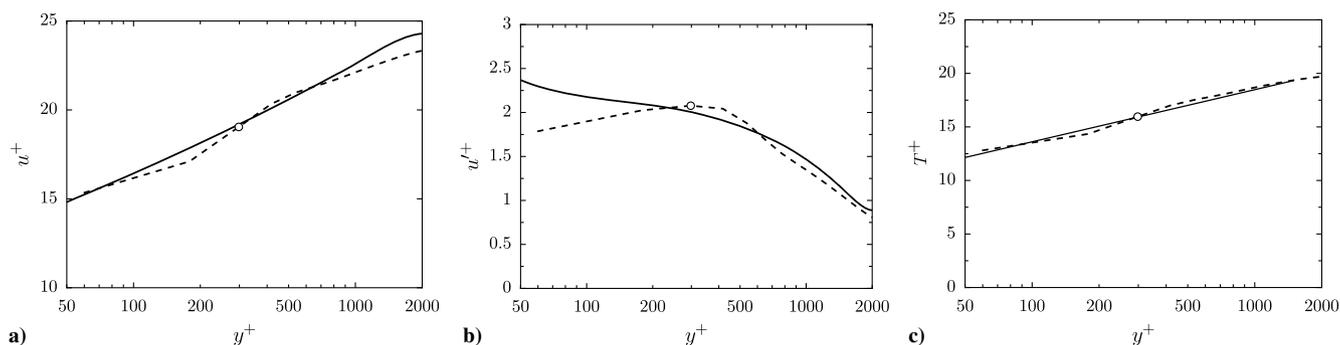
**Fig. 14** Representations of a) mean and b) rms streamwise velocities: LES (dashed lines), and DNS of [32] (solid lines); and c) mean temperature: LES (dashed line) and Kader's law [29] (solid lines).
