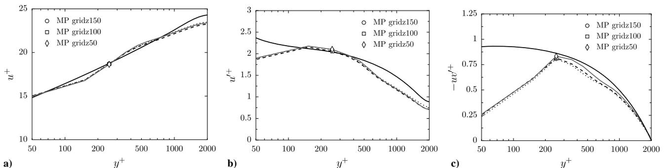
**Fig. 12** Representations of a) mean streamwise velocities, b) rms streamwise velocities, and c) Reynolds shear stresses: LESs using gridz150 (dotted lines), gridz100 (dashed lines), and gridz50 (grey, solid lines); DNS of [32] (black, solid lines).
