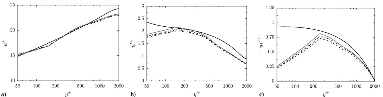
Fig. 10 Representations of a) mean streamwise velocities, b) rms streamwise velocities, and c) Reynolds shear stresses: LESs G1 (dashed–dotted lines), G2 (dashed lines), G3 (grey, solid lines), and G4 (dotted lines); DNS of [32] (black, solid lines).
