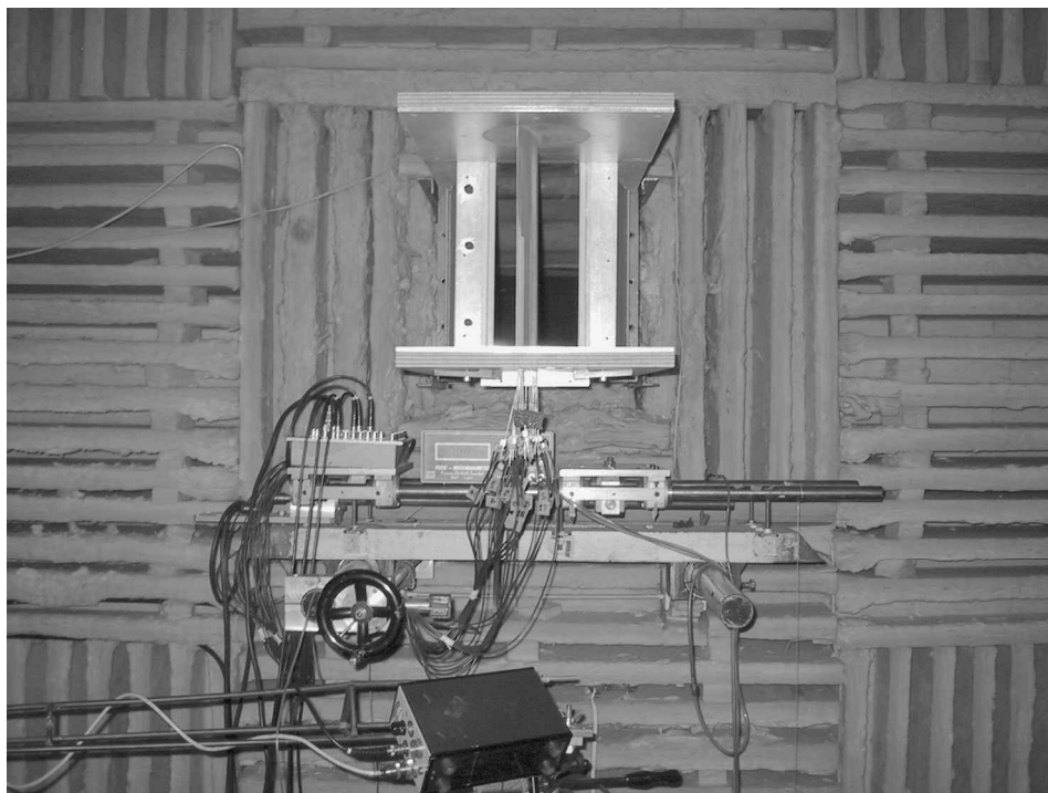
Fig. 1 Experimental setup with the Valeo profile in the ECL test facility.
