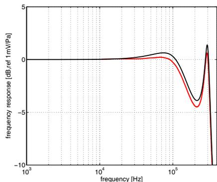
Figure 6: Red line: Amplitude of the frequency response  $|\tilde{H}(f)| = |V(f)/P_{th}(f)|$  obtained from a series of recordings at 15 different positions  $r$ . Black line: target response  $|H(f)|$  given in figure 3.
