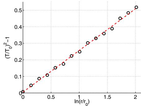
Figure 4: Plot of the evolution of the half duration  $T$  with the propagation distance in order to estimate the initial pressure level at the distance  $r_0$ .
