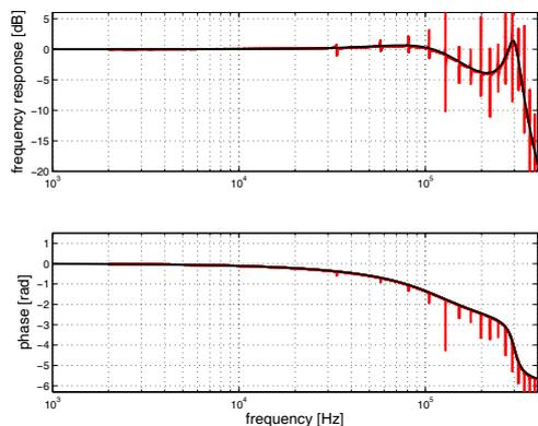
Figure 5: Frequency response  $\tilde{H}(r, f) = V(f, r)/P_{th}(f, r)$  estimated from measured and simulation data at the distance  $r = 356$  mm from the spark source.
