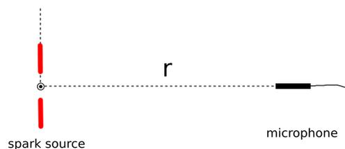
Figure 1: The calibration method is based on the measurement of  $N$ -waves at distances  $r$  from tens of centimeters to  $1.5 \text{ cm}$  from a spark source.
