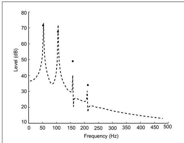
Figure 16. Computed acoustic spectrum.  $U_0 = 11$  m/s;  $\xi = 0.45$ . Same conditions as in the experiment of Figure 13a. Black dots stand for the measured peak values.
