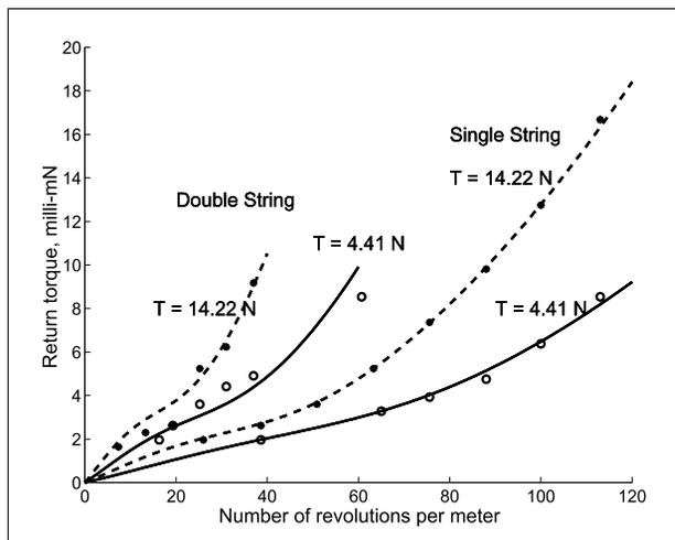
Figure 15. Return torque as a function of twist, for strings made of vegetal fibers.
