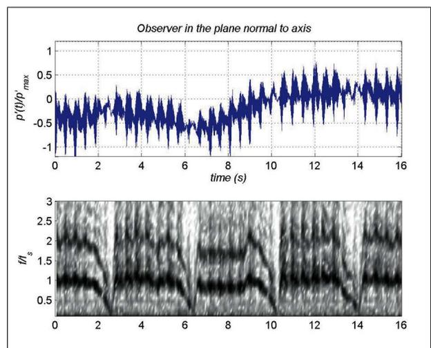
Figure 2. Typical analysis of bullroarer sound, as measured normal to the whirl axis. Top: acoustic pressure signal scaled by its maximum amplitude. Bottom: time-frequency plot; frequency made non-dimensional by the dominant spinning frequency  $f_s$ .
