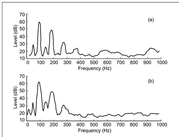
Figure 14. Sound spectra measured on the whirl axis (a) and normal to the axis (b) for a bullroarer with ball bearings in stabilized autorotation.
