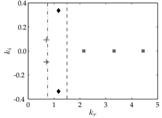
FIGURE 2 – Symmetric modes of the vortex sheet model for the case  $\omega = 0.5$ ,  $\rho_\infty = 1$  and  $M_j = 3$ , + Kelvin - Helmholtz symmetric mode,  $\blacklozenge$  first acoustic mode,  $\blacksquare$  higher acoustic modes,  $---$   $k_r = M_j \omega / (M_j - 1)$ ,  $---$   $k_r = \rho_\infty^{1/2} M_j \omega$ .
