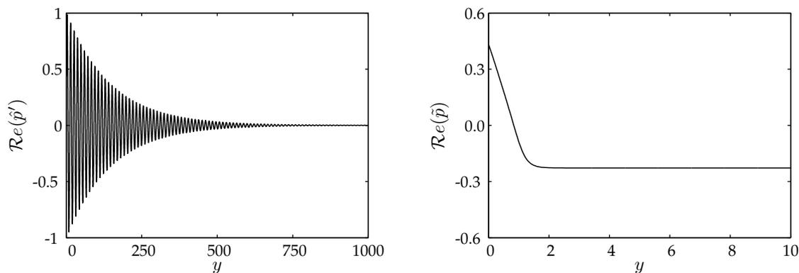
FIGURE 4 – Kelvin - Helmholtz symmetric mode : eigenfunctions  $\tilde{p}$  and  $\hat{p}'$  for  $\delta_\theta = 1/8$ ,  $T_\infty = 1$ ,  $M_j = 3$  and  $\omega = 0.2$ .
