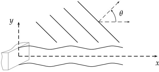
FIGURE 1 – Sketch of Mach wave fronts radiated by a sinuous instability wave, see Eq. (5).
