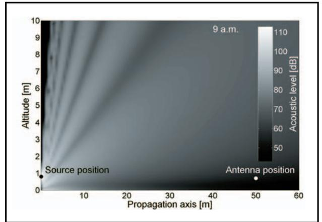
Figure 9. Acoustic levels calculated with a PE code in the propagation plane for case 2 (09/15/99 at 9 a.m.).
