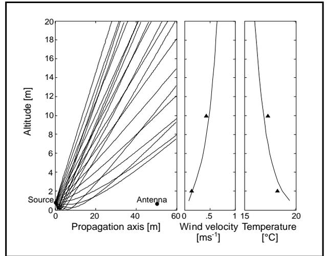
Figure 8. Development of acoustic rays, temperature profiles and wind velocity for case 2 (09/15/99 at 9 a.m.).
