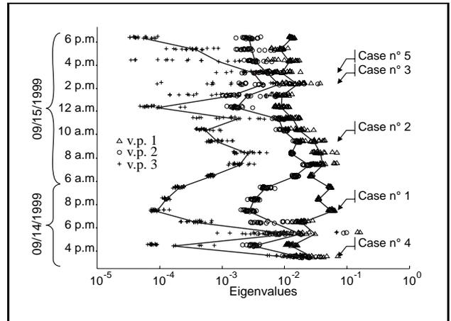
Figure 5. Three greater eigenvalues of correlation matrix on 09/14/99 and 09/15/99, according to time-of-day for an acoustic wave of 930 Hz frequency and 103 dB level, located with an antenna of 1 m length. The solid lines are the mean values of the eigenvalues.
