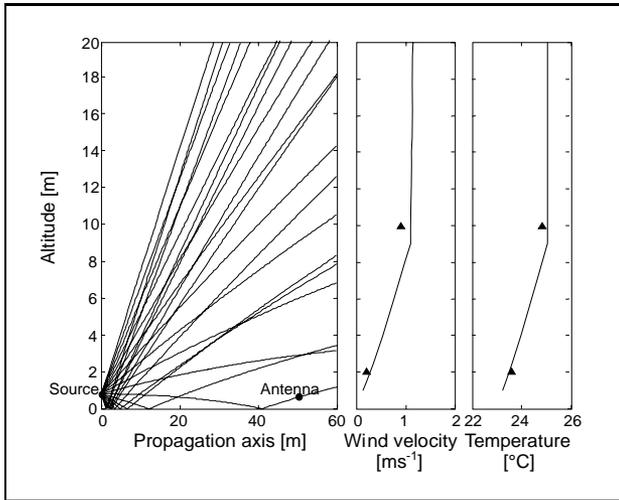
Figure 6. Development of acoustic rays, temperature profiles and wind velocity for case 1 (09/14/99 at 7 p.m.).
