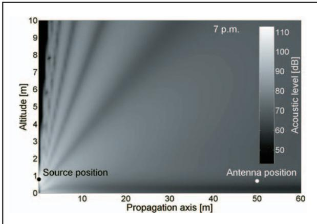
Figure 7. Acoustic levels calculated with a PE code in the propagation plane for case 1 (09/14/99 at 7 p.m.).
