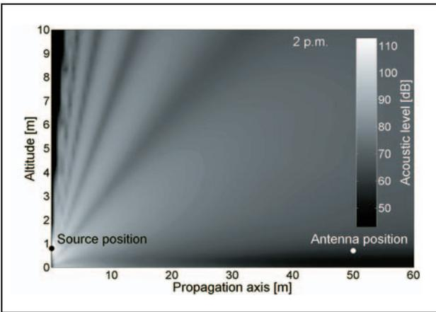
Figure 11. Acoustic levels calculated with a PE code in the propagation plane for case 3 (09/15/99 at 2 p.m.).
