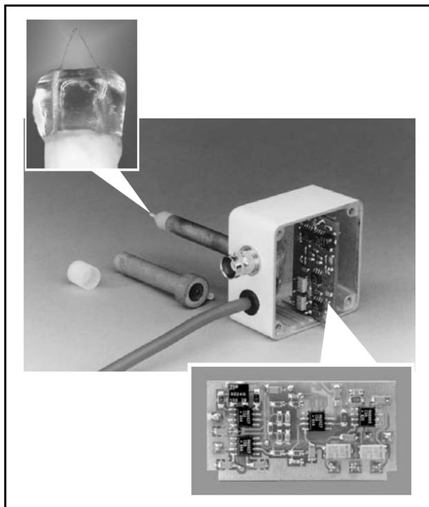
Figure 2. View of the amplification module ( $\times 500\,000$ ) and of the thermocouple of  $1.27 \mu\text{m}$ .
