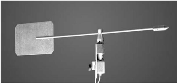
Figure 3. "Autonomous" wind vane.
