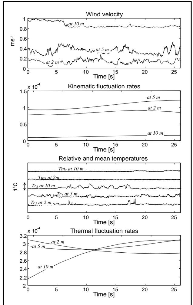
Figure 12. Wind velocity and temperature measurements as a function of time at three heights for case 1 (09/14/99 at 7 p.m.),  $T_m$  is the mean temperature and  $Tr_i$  is the relative temperature.
