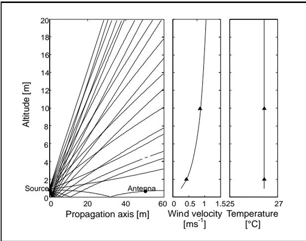
Figure 10. Development of acoustic rays, temperature profiles and wind velocity for case 3 (09/15/99 at 2 p.m.).
