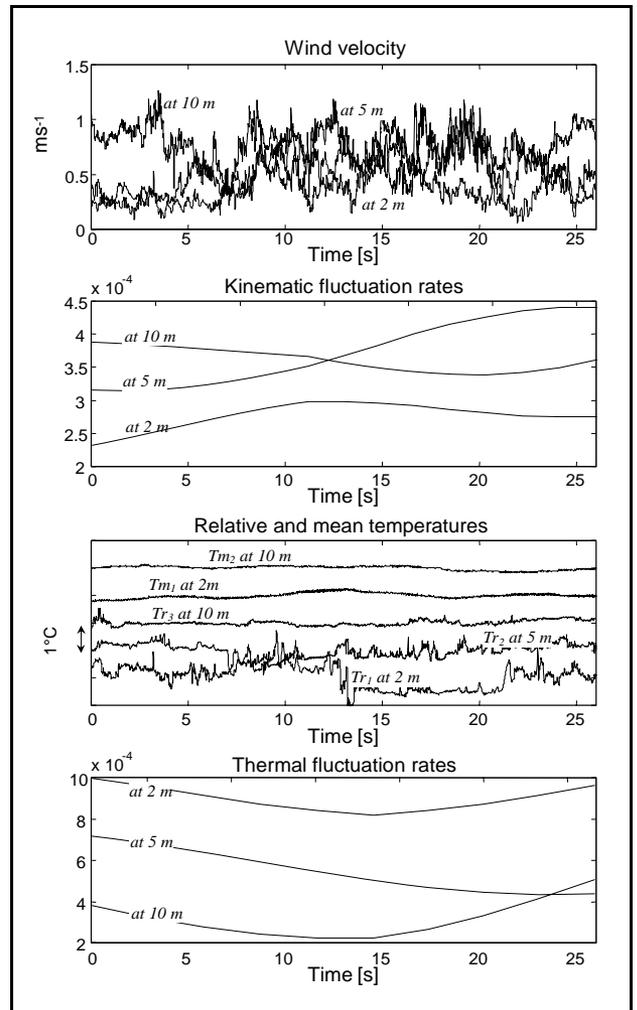
Figure 14. Wind velocity and temperature measurements as a function of time at three heights for case 3 (09/15/99 at 2 p.m.),  $T_m$  is the mean temperature and  $Tr_i$  is the relative temperature.
