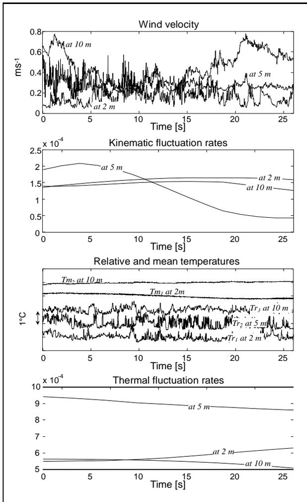
Figure 13. Wind velocity and temperature measurements as a function of time at three heights for case 2 (09/15/99 at 9 a.m.),  $T_m$  is the mean temperature and  $Tr_i$  is the relative temperature.
