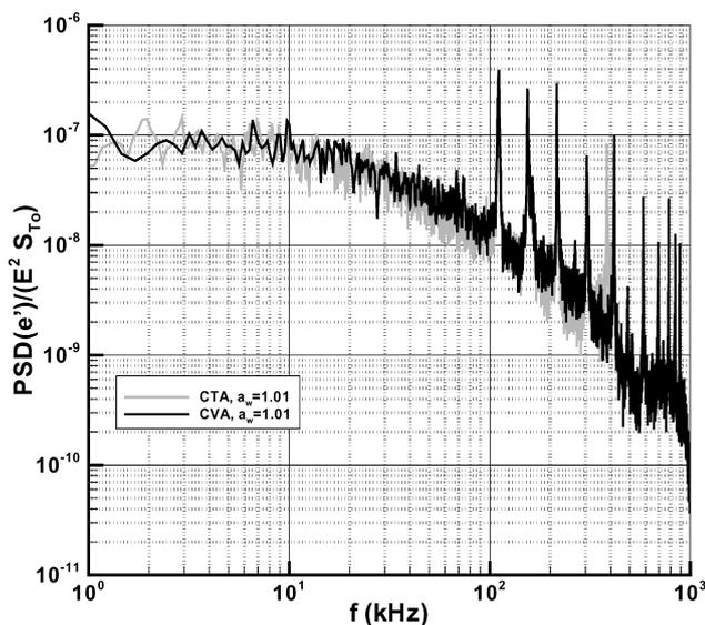
Fig. 3 Comparison of CTA and CVA spectra with respective software corrections ( $y/\delta = 0.36$ ).
