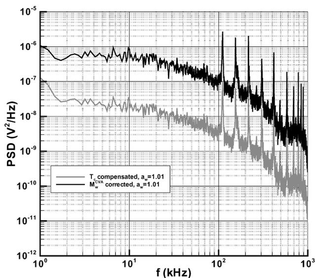
Fig. 2 Partial hardware  $T_c$  compensated and full software  $M_w^{CVA}$  corrected CVA spectra ( $y/\delta = 0.36$ ).
