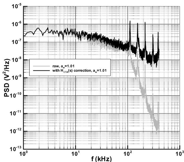
Fig. 1 Raw CTA spectra and corrected CTA spectra ( $y/\delta = 0.36$ ).
