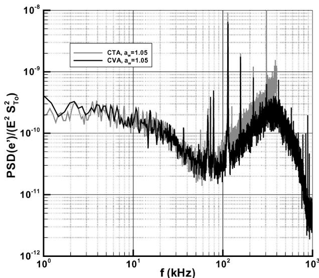
Fig. 4 Comparison of CTA and CVA spectra with respective software corrections (freestream measurements:  $y/\delta = 1.5$ ).
