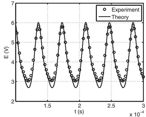
Figure 7. Response of the DISA 55M10 to a sinusoidal perturbation of amplitude  $A_t = 200$  mV and frequency  $f_i = 27$  kHz.
