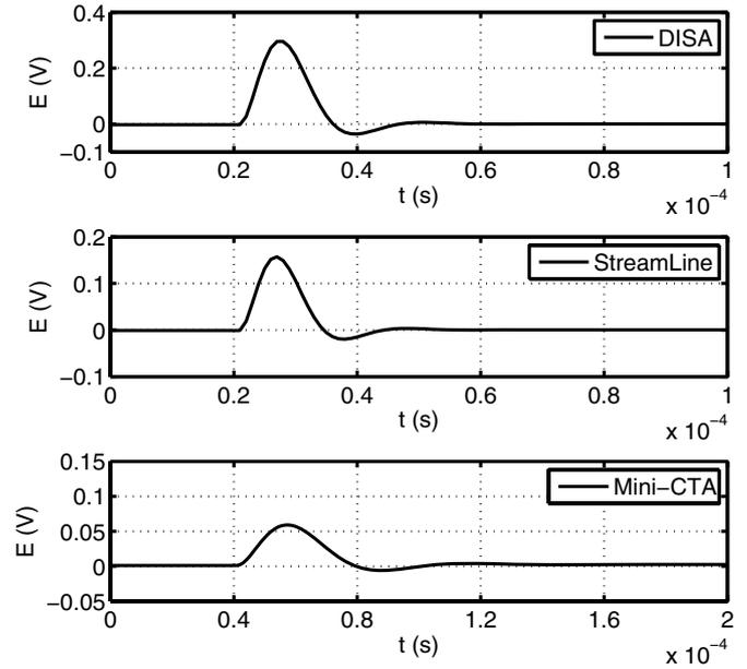
**Figure 4.** Simulated square-wave responses of the CTAs. Note the different time scales.
