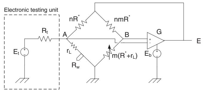
Figure 1. Schematic diagram of a CTA.
