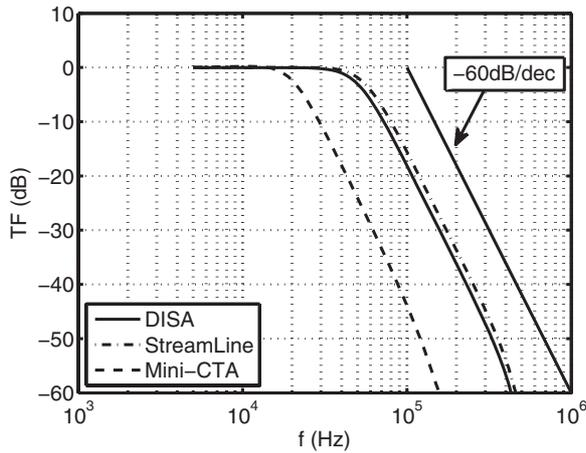
Figure 5. Amplitude transfer function of the simulated CTA models.
