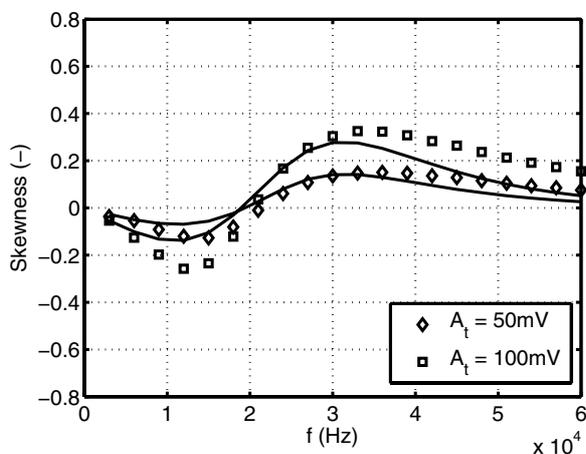
**Figure 9.** Skewness factor, StreamLine. Symbols: experiments; solid lines: theory.
