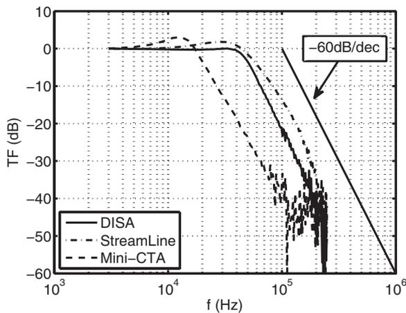
**Figure 3.** Amplitude transfer function of the CTAs.
