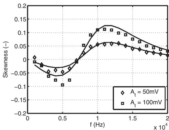
**Figure 10.** Skewness factor, Mini-CTA. Symbols: experiments; solid lines: theory.
