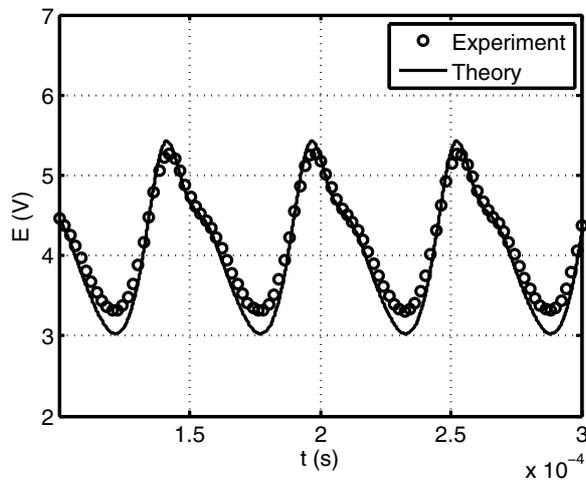
Figure 6. Response of the DISA 55M10 to a sinusoidal perturbation of amplitude  $A_t = 200$  mV and frequency  $f_i = 18$  kHz.
