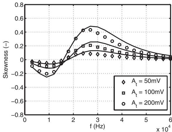
**Figure 8.** Skewness factor, DISA 55M10. Symbols: experiments; solid lines: theory.
