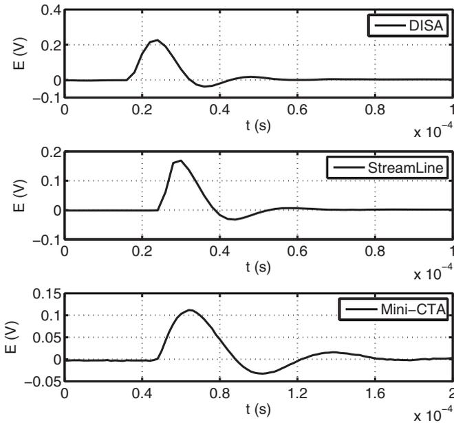
**Figure 2.** Experimental square-wave responses of the CTAs. Note the different time scales.
