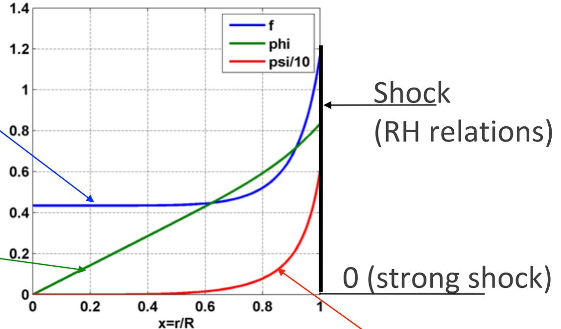
$$v(r, t) = c_0 \left( \frac{R_0}{R(t)} \right) \phi \left( \frac{r}{R(t)} \right)$$
