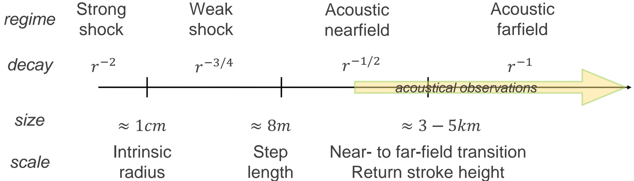
We developed (*Lacroix et al. GRL, 2019*) a new model based on *Few (1969, 1995)* model to explain the full acoustic spectrum and its variability with distance. It takes into account three components:
