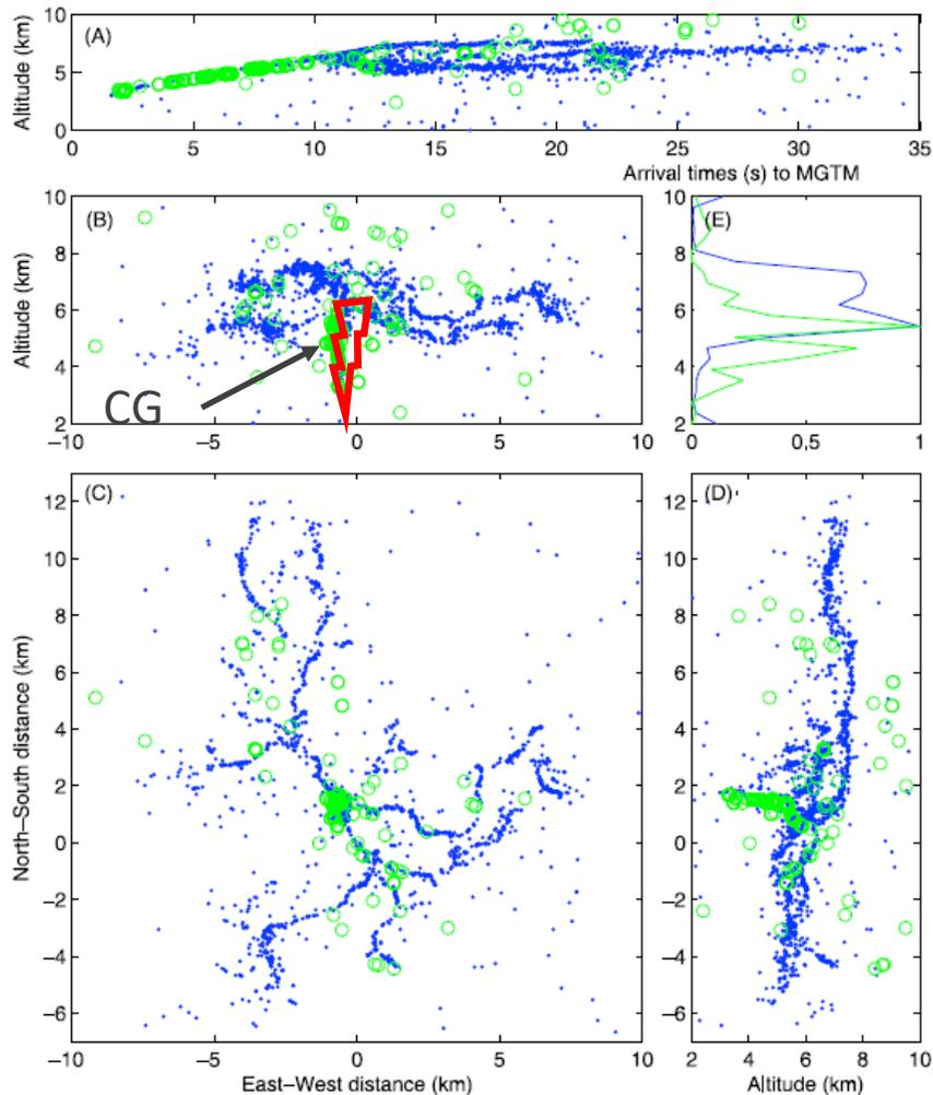
Figure 7. Overlays of locations of acoustical (circles) and LMA radiation sources (dots) for the second triggered lightning flash over the triggering site (Kiva) on the Magdalena Mountains of New Mexico at 2322:48 UTC on 6 August 2009. See Figure 6.
