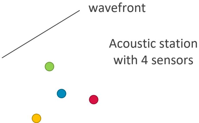
Considering that the source is far enough to have a plane wavefront, the PMCC algorithm - Progressive Multi-Channel Correlation (*Cansi, 1995; Cansi and Le Pichon, 2008*) - can give the azimuth and apparent ground speed (projection of the wave speed in the plane of the sensors).
