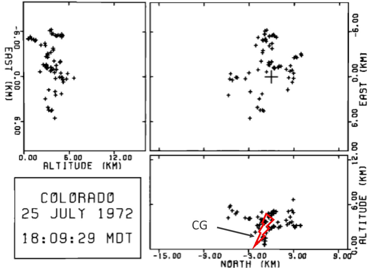
⑨ First 3D view of the discharges **inside** the cloud (EM methods under development at that time) so no external validation of these results.
