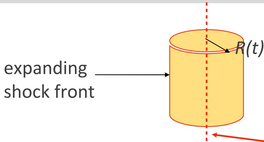
Single driving parameter : **deposited energy / unit length** [J/m]  $E_0$
