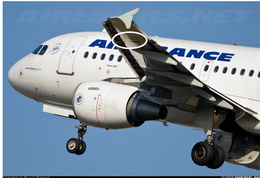
fuel pressure relief vent on a A319
