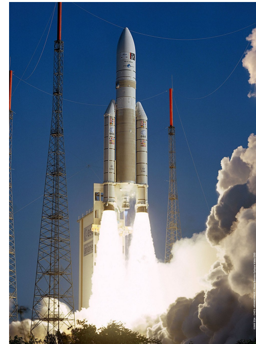
Ariane V, M = 780 tons, 2 solid boosters P230 providing 92% of the lift-off thrust
