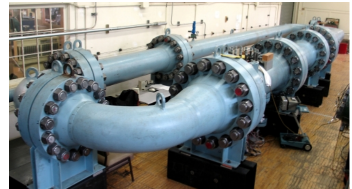
McKeon et al. (2004) - Superpipe , the Reynolds number is increased through the pressure
