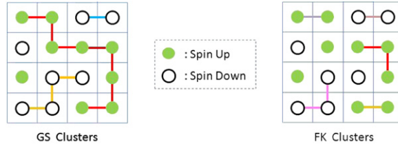
Fig. 13. Illustration of GS clusters (left) versus FK clusters (right) for an Ising spin configuration. Different distinct clusters are shown in different colors. A GS cluster in a spin configuration, is a set of nearest-neighbor sites of like states. An FK cluster can then be constructed from a GS cluster by randomly assigning a bond between each pair of spins with a temperature dependent probability p := 1 - e^{-2\beta} . The critical point on the square lattice is at \beta_c = \frac{1}{2} \ln(1 + \sqrt{2}) and p_c = \sqrt{2}/(1 + \sqrt{2}) . (For interpretation of the references to color in this figure legend, the reader is referred to the web version of this article.)
