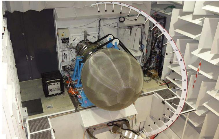
FIGURE 2 – Characterization of fan noise in the ECL-B3 facility (1/3 scale of a real engine) at Ecole Centrale de Lyon.
