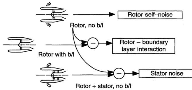
FIGURE 1 – As an illustration, experimental protocol for the extraction of the noise associated with different sub-components of a rotating machine, from Ganz *et al.*<sup>4</sup>
