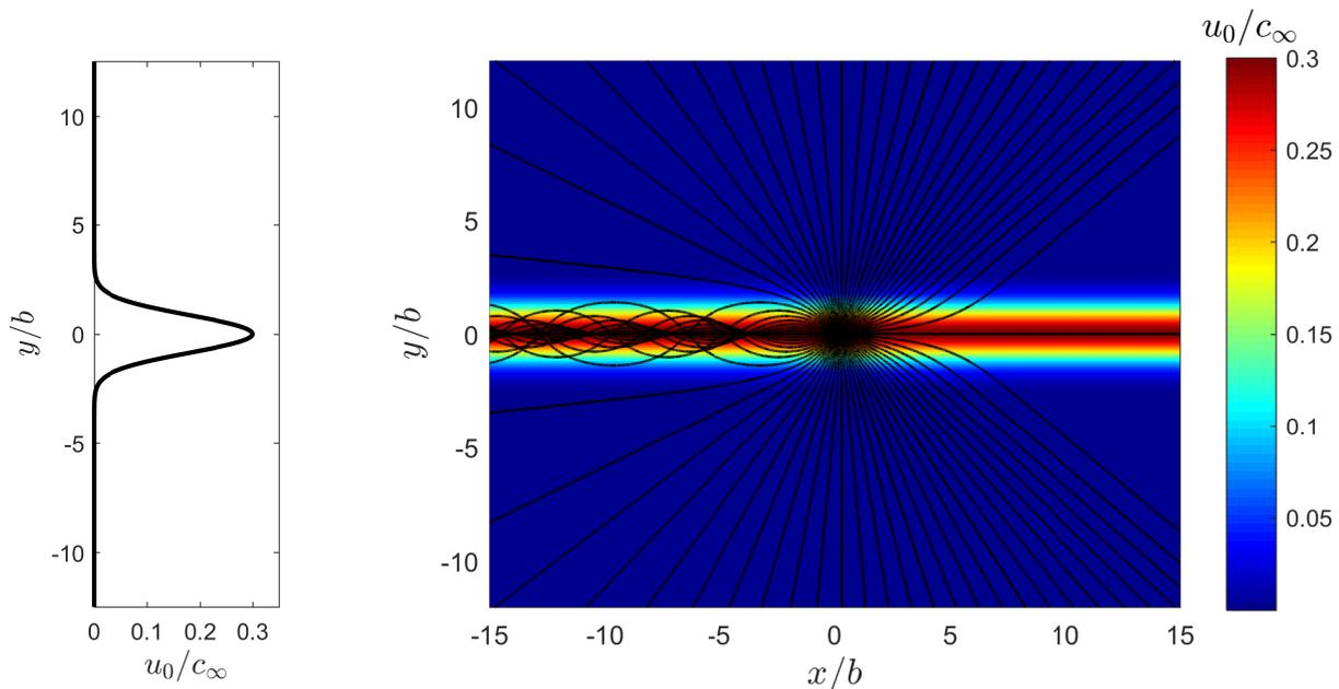
FIGURE 1 – Ray paths through a jet with a Gaussian velocity profile, for a point acoustic source located at  $(x_s, y_s) = (0, 0)$ . We can observe refraction effects bending the rays when they travel through the jet. We can also notice that some rays propagating towards  $x < 0$  are trapped within the jet, acting as a waveguide.
