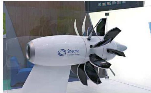
Snecma's SAGE 2 demonstrator is planned for flight testing on a modified A340-600 in 2016.
