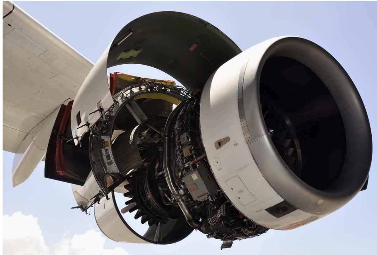
Close-up of a CFM56-5C engine powering the Airbus A340 airliner.
