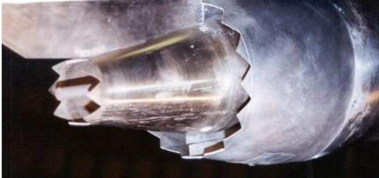
High-bypass-ratio nozzle (cfm56 type)
