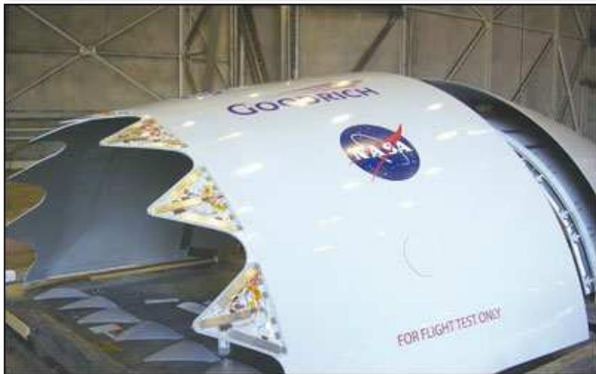
A look at the inner workings of the variable-geometry chevron. Each chevron includes three nickel-titanium actuators.
