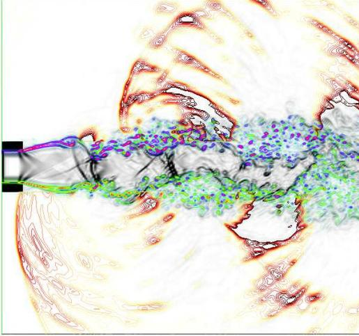
Figure 4: Computation of the generation of screech tones in an underexpanded supersonic jet, fully expanded jet at Mach number 1.55, Reynolds number  $6 \times 10^4$ . Snapshot of the density modulus, of the spanwise vorticity and of the near-field pressure, in a plane perpendicular to the spanwise direction. The nozzle lips are represented in black. From Berland *et al.* (2007).
