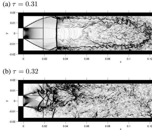
Figure 8: Compressible large-eddy simulation of the turbulent flow behind a sudden enlargement of rectangular duct cross-section: snapshot of density gradient  $|\nabla\rho|$  for two pressure ratios for the case  $L = 0.16$  m,  $L/H = 5.23$  and  $h/H = 0.3$ . See Emmert *et al.* (2007).
