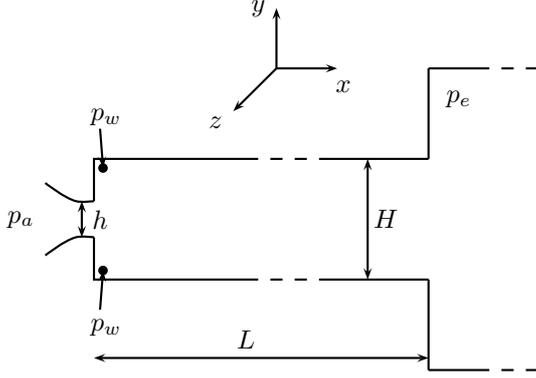
Figure 6: Sudden enlargement of rectangular duct cross-section: the flow regime is characterized by the pressure ratio between the plenum chamber and the reservoir pressure  $\tau = p_e/p_a$ . The area ratio is given by  $h/H$ , where  $h$  is the nozzle height and  $H$  the height of the test-duct;  $L$  is the duct length and  $b$  is the width of the nozzle and of the duct. The flow can be monitored by the base pressure  $p_w$  at the two upstream corners of the channel.
