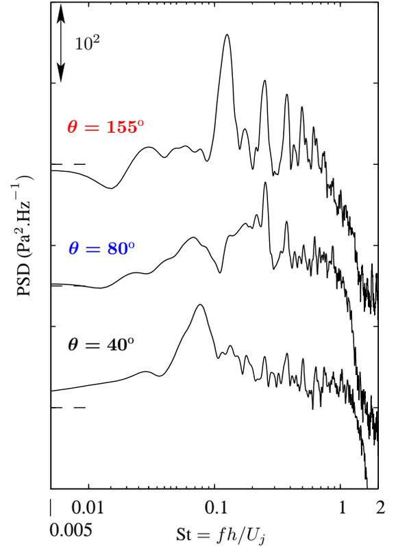
Figure 5: Computation of the generation of screech tones in an underexpanded supersonic jet, fully expanded at jet Mach number 1.55, Reynolds number  $6 \times 10^4$ . From Berland *et al.* (2007).
