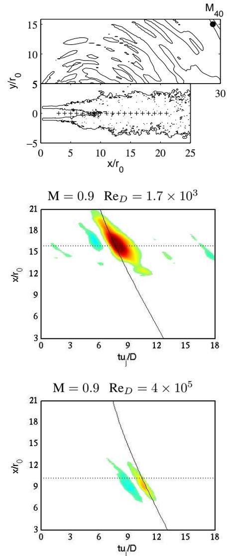
Figure 3: Correlation coefficient  $C_{\omega p}(x/r_0, tu_j/D)$  between the vorticity along the jet axis at  $\mathbf{x}_1 = (x, 0, 0)$  and the acoustic field at  $\bullet \mathbf{x}_2 = M_{40}$ . Time delay  $tu_j/D$  versus axial distance  $x/r_0$ , — time of propagation at the speed of sound, ..... end of the potential core  $x = x_c$ , color scale:  $[-0.14 \ 0.14]$  (white:  $[-0.035 \ 0.035]$ ).
