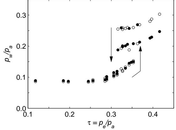
Figure 7: Turbulent flow behind a sudden enlargement of rectangular duct cross-section for the case  $L = 0.16$  m,  $L/H = 5.23$  and  $h/H = 0.3$ . Experimental data of the upper  $\circ$  and lower  $\bullet$  normalized mean base pressure  $p_w/p_a$  as a function of the pressure ratio  $\tau$ , from Anderson *et al.* (1977).
