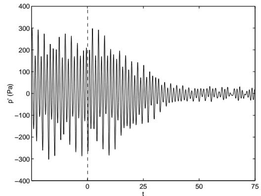
Figure 10: Numerical simulation of a closed-loop active control in a 3-D cavity. Time evolution of the pressure radiated at point  $P$ , see Fig. 9, before and after control. Control phase starts at  $t = 0$ . From Marsden *et al.* (2003).
