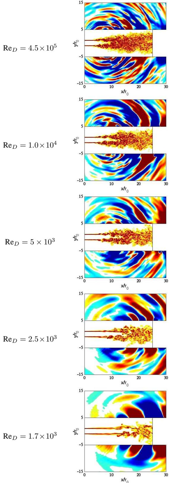
Figure 2: Jets at Mach  $M = 0.9$ . Snapshots of the vorticity norm  $|\omega|$  in the flow and of the fluctuating pressure  $p'$  outside, in the plane  $z = 0$ . For the five simulations, the color scale of the vorticity norm is  $|\omega| \times r_0 / u_j = [0, 2.65]$ , and the pressure color scale is  $p' = [-70, 70]$  Pa or  $p' / (\rho_j u_j^2) = [-6.2, 6.2] \times 10^{-4}$ .
