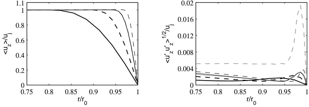
Figure 2. Profiles at  $z = 0$  of mean axial velocity  $\langle u_z \rangle$ , and of the rms values of fluctuating axial velocity  $u'_z$ , for: — JetD02, - - - JetD01, ——— JetD005, - · - · JetD0025, ····· JetD005p250, - - - JetD005p2000.
