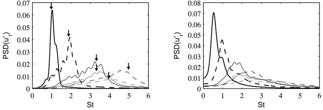
Figure 12. Spectra of velocity  $u'_r$  obtained at  $r = r_0$ , as functions of Strouhal number  $St = fD/u_j$ . Left, around rolling-up at  $z = z_{roll}$ , right, just downstream of pairing at  $z = z_{pair}$ , for: — JetD02, - - - JetD01, — JetD005, - - - JetD0025, — JetD005p250, - - - JetD005p2000 ( $z_{roll}$  and  $z_{pair}$  are given in table 5). The arrows indicate the frequencies determined from the initial momentum thickness using  $f\delta_\theta/u_j = 0.012$ .
