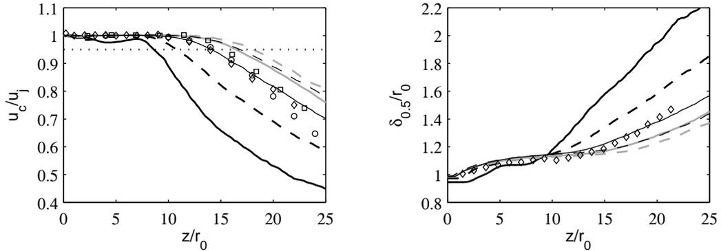
Figure 13. Variations of centerline mean axial velocity  $u_c$  and of jet half-width  $\delta_{0.5}$ , for: — JetD02, - - - JetD01, — JetD005, - - - JetD0025, — JetD005p250, - - - JetD005p2000 (the dotted line represents  $u_c = 0.95u_j$ ). Measurements:  $\circ$  Lau *et al.*,<sup>32</sup>  $\square$  Arakeri *et al.*,<sup>33</sup>  $\diamond$  Fleury *et al.*<sup>34</sup>
