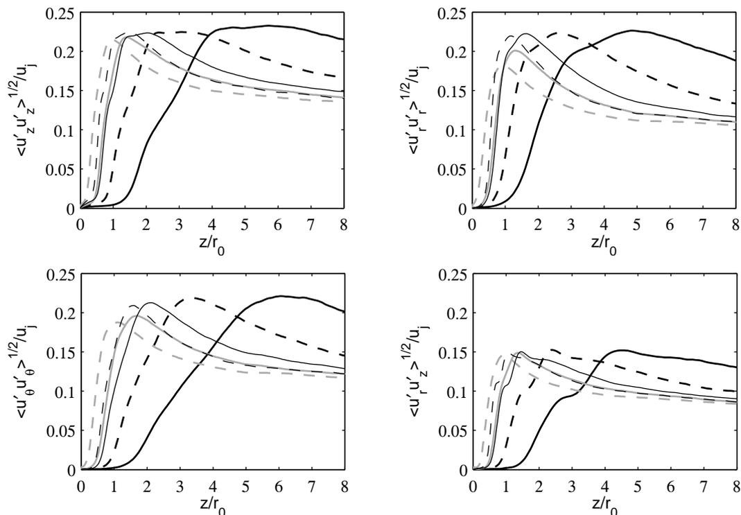
Figure 11. Variations along the lip line at  $r = r_0$  of the rms values of fluctuating velocities  $u'_z$ ,  $u'_r$  and  $u'_\theta$ , and of the magnitude of Reynolds stress  $\langle u'_r u'_z \rangle$ , for: — JetD02, - - - JetD01, — JetD005, - - - JetD0025, — JetD005p250, - - - JetD005p2000.
