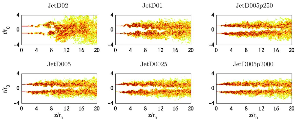
Figure 6. Snapshots in the  $(z, r)$  plane of vorticity norm. The color scale ranges up to the level of  $6.5u_j/r_0$ .
