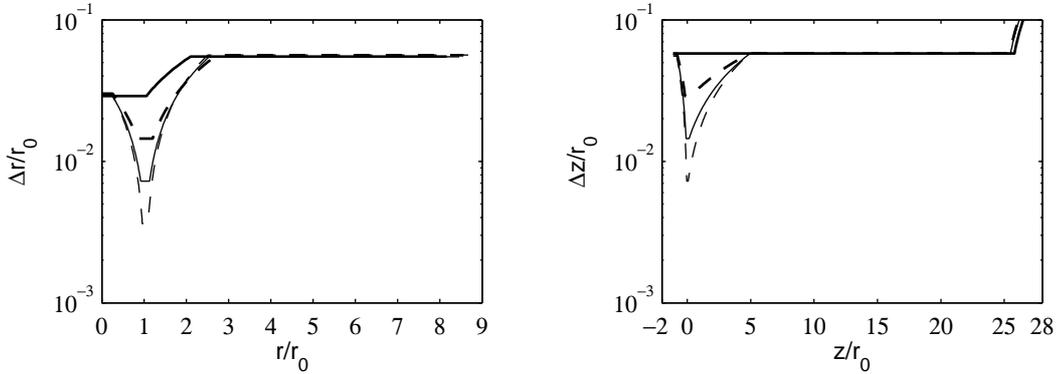
**Figure 1.** Mesh spacings in the radial and axial directions,  $\Delta r$  and  $\Delta z$ , in the LES, for: — JetD02, - - JetD01, ··· JetD005, - · - JetD0025, ——— JetD005p250, - - - JetD005p2000.
