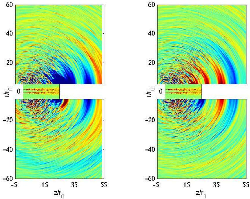
Figure 9. Snapshots in the  $(z, r)$  plane of the pressure field obtained from the acoustical simulations for JetD005p2000, using the full control surface (left) and a control surface limited to  $z \leq z_c + 2r_0$  (right), where  $z_c$  is the position of the potential core end. The color scales range from -40 to 40 Pa for pressure, and up to  $8u_j/r_0$  for vorticity norm in the LES jet flow.
