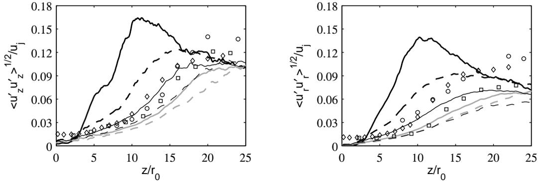
**Figure 14.** Variations along the centerline at  $r = 0$  of the rms values of fluctuating velocities  $u'_z$  and  $u'_r$ , for: **—** JetD02, **- - -** JetD01, **—** JetD005, **- - -** JetD0025, **—** JetD005p250, **- - -** JetD005p2000. Measurements:  $\circ$  Lau *et al.*,<sup>32</sup>  $\square$  Arakeri *et al.*,<sup>33</sup>  $\diamond$  Fleury *et al.*<sup>34</sup>
