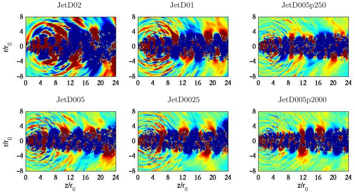
Figure 8. Snapshots in the  $(z, r)$  plane of the fluctuating pressure obtained by LES. The color scale ranges for levels from -250 to 250 Pa.
