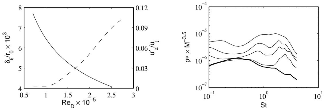
Figure 5. Experimental results by Zaman.<sup>7,8</sup> Left: variations of nozzle-exit, — boundary-layer momentum thickness  $\delta_\theta$  and - - - maximum turbulent intensity  $u'_z/u_j$ , with Reynolds number  $\text{Re}_D$  for untripped jets. Right: far-field pressure spectra at  $90^\circ$  for, — untripped jets at  $\text{Re}_D = 0.7 \times 10^5$ ,  $0.8 \times 10^5$ ,  $10^5$  and  $1.3 \times 10^5$  (from top to bottom) and — a tripped jet at  $\text{Re}_D = 1.3 \times 10^5$ .
