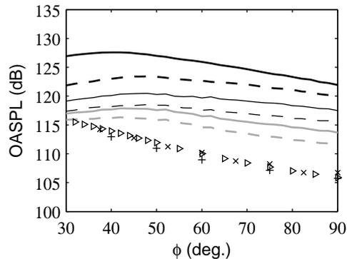
Figure 16. Sound pressure levels obtained at  $60r_0$  from the jet nozzle exit, as functions of the radiation angle relative to the jet direction, for: — JetD02, - - - JetD01, — JetD005, - - - JetD0025, ··· JetD005p250, - · - JetD005p2000. Measurements: + Mollo-Christensen *et al.*,<sup>35</sup> × Lush,<sup>36</sup> < Tanna,<sup>37</sup> > Bogey *et al.*<sup>38</sup>
