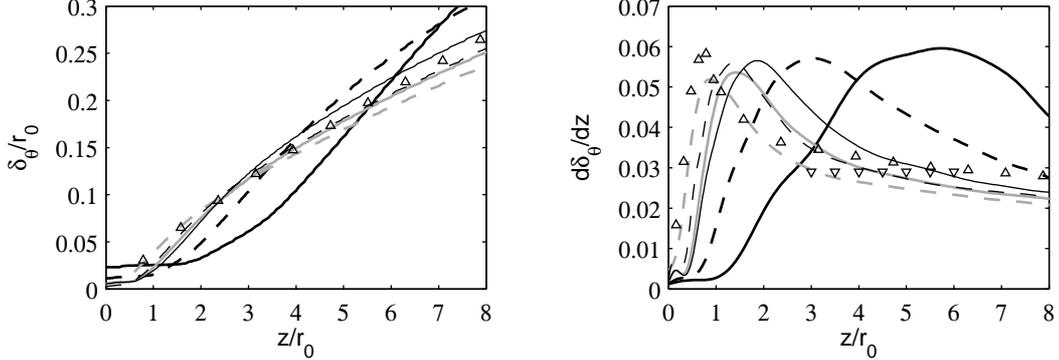
Figure 10. Variations of shear-layer momentum thickness  $\delta_\theta$ , and of spreading rate  $d\delta_\theta/dz$ , for: — JetD02, - - - JetD01, ——— JetD005, - - - - JetD0025, ——— JetD005p250, - - - - JetD005p2000. Measurements:  $\nabla$  Hussain and Zedan,<sup>4</sup>  $\triangle$  Husain and Hussain.<sup>6</sup>
