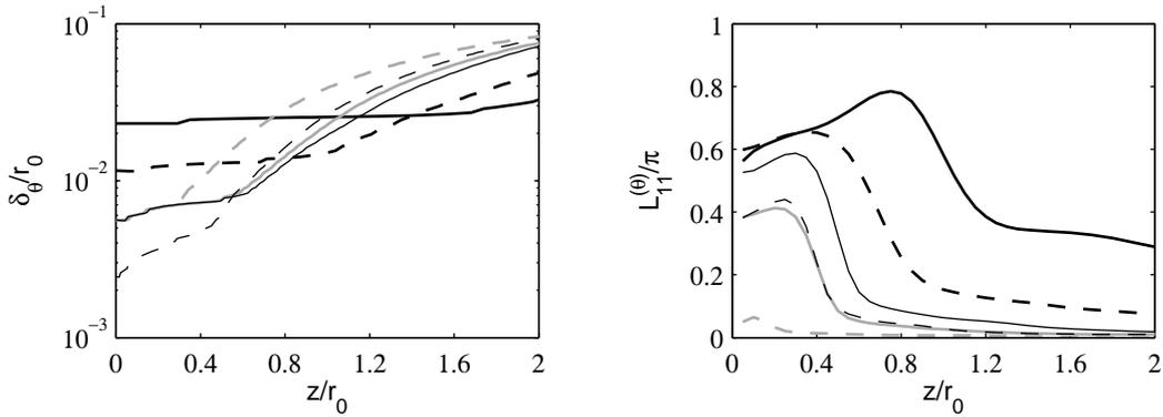
**Figure 3.** Axial variations in the vicinity of the pipe lip, of the shear-layer momentum thickness  $\delta_\theta$ , and of the integral length scale in the azimuthal direction  $L_{11}^{(\theta)}$  calculated from the fluctuating axial velocity at  $r = r_0$ , for: — JetD02, - - - JetD01, ——— JetD005, - · - · JetD0025, ——— JetD005p250, - - - JetD005p2000.
