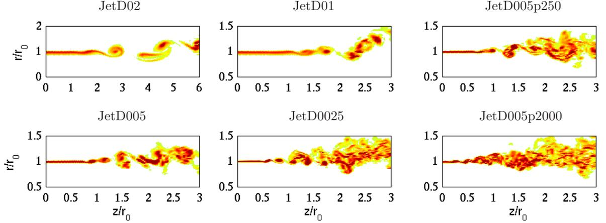
Figure 7. Snapshots in the  $(z, r)$  plane of vorticity norm downstream of the pipe lip. The color scale ranges up to the level of  $10u_j/r_0$  for JetD02, but up to  $20u_j/r_0$  for the other jets.
