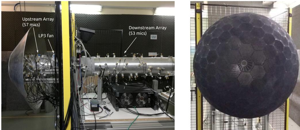
Figure 3. Left : Inlet (without the TCS) and instrumented duct. Right : Turbulence Control Screen (TCS). The fan can be seen through the honeycomb.
