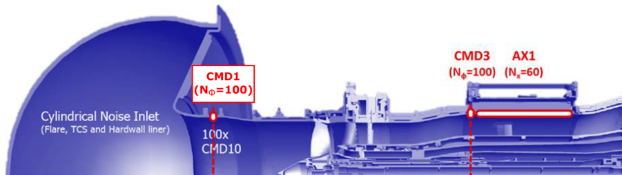
Fig. 1 Sketch of the fan rig showing the in-duct microphone arrays.
