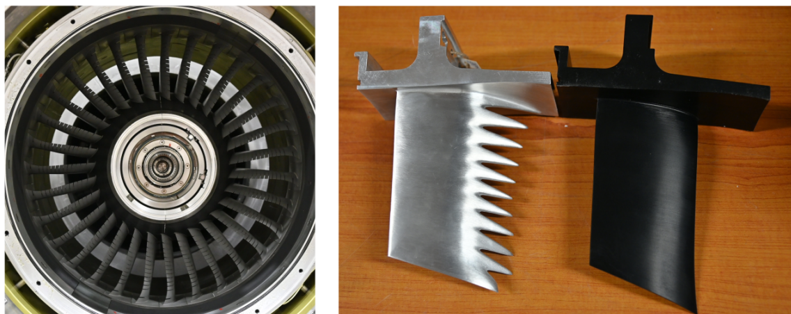
Fig. 3 Low-noise OGVs with leading edge features. Slitted OGV mounted on the test-rig without the fan blades (left) and serrated OGV compared to the baseline OGV with straight leading edge (right).
