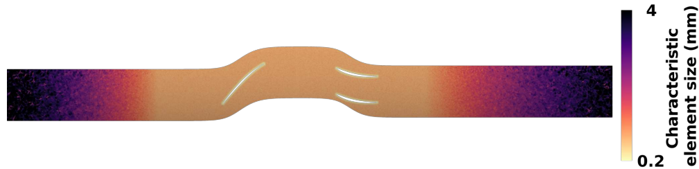
Fig. 2 Radial cut of the computational domain colored by the element characteristic size.
