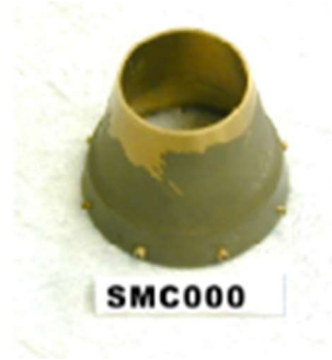
Figure 1: Baseline Small Metal Chevron (SMC000) Nozzle.
