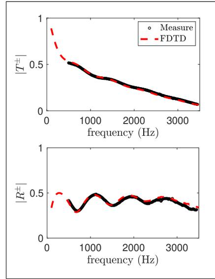
**Figure 2.** Comparison of the transmission and reflection coefficients of the FDTD code with the experimental results of Aurégan and Singh [13] for a Nickel-Chrome alloy foam ( $\phi = 0.99, \alpha_\infty = 1.17, \Lambda = 1.0 \cdot 10^{-4}$  m,  $\Lambda' = 2.4 \cdot 10^{-4}$  m), corresponding to a cavity length of 200 mm and a depth of 25 mm.
