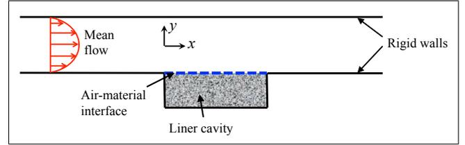
Figure 1. Sketch of the geometry of the 2D lined duct.
