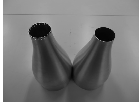
Fig. 1 Photograph of the notched nozzle (left) and the baseline nozzle (right).
