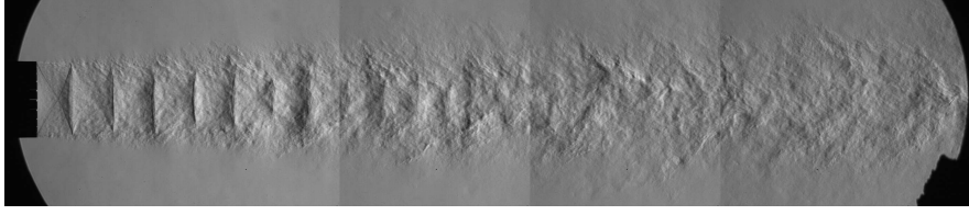
Figure 1. Schlieren image of a jet at M_j = 1.10 . The picture is made up of five uncorrelated spark images (exposure time of 4 \mu\text{s} ) recorded at different axial locations.
