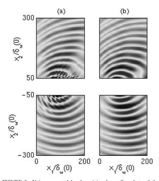
FIGURE 3 Noise generated by the mixing layer. Snapshots of the dilatation field obtained simultaneously: (a) from the LEE (13) with source terms (12), (b) directly from the Navier–Stokes equations. All the calculations are 2-D and quantitative comparisons can be found in Bogey *et al.* (2002a).
