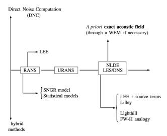
FIGURE 1 Computational aeroacoustics: some methods used for predicting aerodynamic noise. In the direct noise calculation, the aerodynamic field and the acoustic field are obtained in the same computation from DNS, LES, NLDE or URANS, and a wave extrapolation method (WEM) may be used to obtain the far field. In hybrid methods, generation and propagation are split into two distinct steps.
