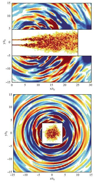
FIGURE 7 LES of a circular jet at M = 0.9 and  $Re_D = 4 \times 10^5$ . Snapshot of the vorticity  $|\omega|$  in the flow and of the fluctuating pressure p' outside. Left: in the x - y plane at z = 0. Right: in the y - z plane at  $x = 11r_0$ . The color scales are from 0 to 8 × 10<sup>4</sup> s<sup>-1</sup> for the vorticity and from -70 to 70 Pa for the pressure. From Bogey and Bailly (2002c).
