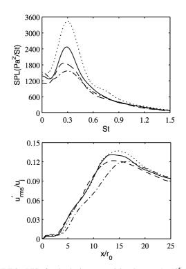
FIGURE 8 LES of a circular jet at M = 0.9 and  $Re_D = 4 \times 10^5$ . Left: sound pressure spectra at  $x = 29r_0$ ,  $r = 12r_0$  in linear scales as a function of the Strouhal number. Right: centerline profiles of the rms-values of the axial fluctuating velocity. LESac \_\_\_\_\_, LESampl ......, LESshear – – – and LESmode –·---. From Bogey and Bailly (2003a).
