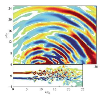
FIGURE 4 Direct computation of noise from LES, circular jet at M = 0.9 and  $Re_D = 6.5 \times 10^4$ , see Bogey *et al.* (2003a) for details. Snapshot of the dilatation field  $\Theta = \nabla \cdot \mathbf{u}$  in the acoustic region, and of the vorticity field  $\omega_z$  in the aerodynamic region, in the x - y plane at z = 0. Note that  $D = 2r_0$ .
