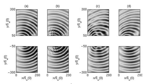
FIGURE 2 Dilatation fields obtained from Lighthill's integral with (a)  $T_{ij}^{f}$  and (c)  $T_{ij}$  as source terms, (b) from the LEE without mean flow, (d) directly from the Navier–Stokes equations. All the calculations are 2-D, and quantitative comparisons can be found in Bogey *et al.* (2003b).
