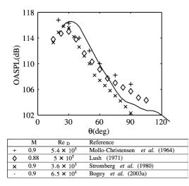
FIGURE 5 Direct computation of noise from LES, circular jet at M = 0.9 and  $Re_D = 6.5 \times 10^4$ , see Bogey *et al.* (2003a) for details. Overall sound pressure level as a function of angle  $\theta$  measured from the jet axis, at  $60r_0$  from the jet nozzle, and comparison with experimental data for different Reynolds numbers.
