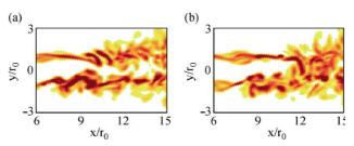
FIGURE 6 Circular jet at M = 0.9 and  $Re_D = 6.5 \times 10^4$ . Snapshot of the vorticity norm  $|\omega|$  in the plane z = 0 (a), at  $t^* = 6.2$ ; (b), at  $t^* = 7.5$ .
