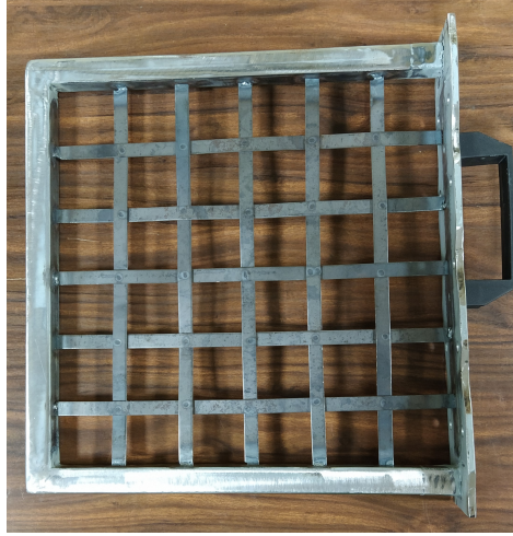
Figure 2.2: Metal grid for turbulence generation with perimeter dimensions 30 cm x 30 cm .
