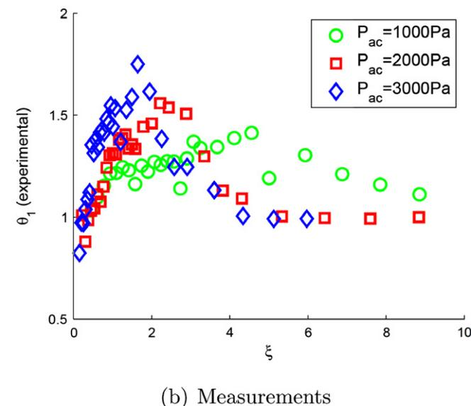
Fig. 4. Amplitudes of temperature fluctuations behind the stack at the fundamental frequency. Top: models. Bottom: measurements. Relaxation parameters used in the model:  $R = 1$  inside the stack,  $R = 10,000$  outside the stack. The hot end of the stack is located at  $\xi = 0$ .
