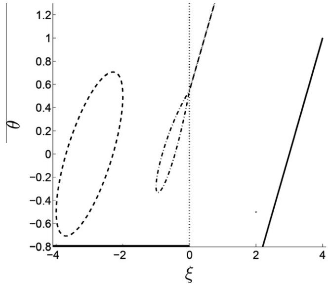
Fig. 1. Position and temperature of three fluid particles during an acoustic cycle. The leftmost particle spends the entire acoustic cycle inside the stack ( $R = 1$  at  $\xi \leq 0$ ). The rightmost particle spends the entire acoustic cycle outside the stack ( $R = \infty$  at  $\xi > 0$ ). The middle particle crosses the edge of the stack. Axial conduction is neglected,  $Pe^{-1} = 0$ .
