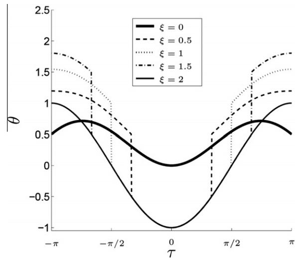
Fig. 2. Temperature fluctuations predicted by the model during an acoustic period at different locations near the stack end.  $R = 1$  inside the stack,  $R = \infty$  outside the stack,  $Pe^{-1} = 0$ .
