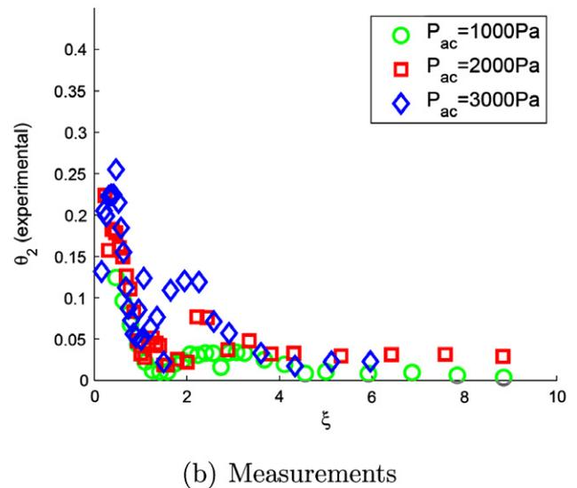
Fig. 5. Amplitudes of temperature fluctuations behind the stack at twice the fundamental frequency. Top: models. Bottom: measurements. Relaxation parameters used in the model:  $R = 1$  inside the stack,  $R = 10000$  outside the stack. The hot end of the stack is located at  $\xi = 0$ .
