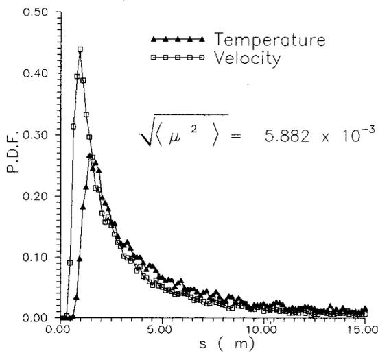
**Figure 7.** Probability density of distance to the first caustic: comparison between a scalar case and a vectorial case with the same r.m.s. value of the index of fluctuation  $\sqrt{\langle \mu^2 \rangle}$ .
