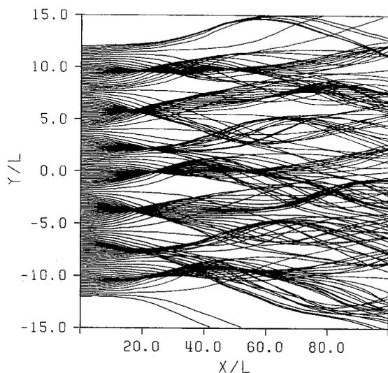
**Figure 1.** Ray-tracing through a single realization of a two-dimensional isotropic scalar field ( $\theta/T_0 = 1.176 \times 10^{-2}$ ,  $L = 0.1$  m).
