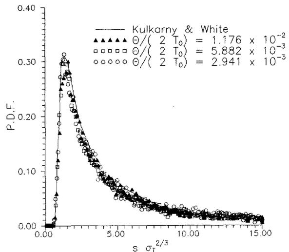
**Figure 4.** Rescaling of the probability densities curves in terms of the Kulkarny and White parameter  $\sigma_T$  for two-dimensional scalar fields.
