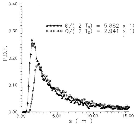
**Figure 3.** Probability densities of distances to the first caustic for two-dimensional scalar fields ( $L = 0.1$  m).
