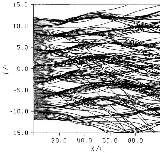
**Figure 5.** Ray-tracing through a single realization of a two-dimensional isotropic vectorial field ( $v'/c_0 = 5.882 \times 10^{-3}$ ,  $L = 0.1$  m).
