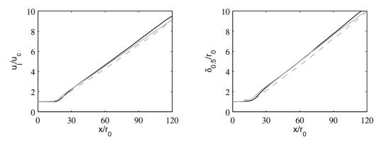
FIG. 4 – Variations of the inverse of centerline mean axial velocity  $u_j/u_c$  (left) and of the jet half-width  $\delta_{0.5}/r_0$  (right), for : — jetRe3600, — jetRe3600thin, and – – jetRe3600mode.
