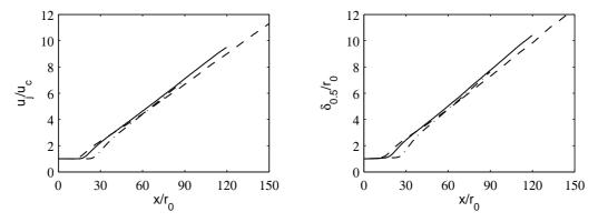
FIG. 3 – Variations of the inverse of centerline mean axial velocity  $u_j/u_c$  (left) and of the jet half-width  $\delta_{0.5}/r_0$  (right), for :  $-\cdot - \cdot$  jetRe1800, — jetRe3600, and - - jetRe11000.
