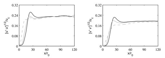
FIG. 6 – Variations along the jet centerline of axial and radial turbulence intensities  $[u'u']^{1/2}/u_c$  (left) and  $[v'v']^{1/2}/u_c$  (right), for : — jetRe3600, — jetRe3600thin, and – – jetRe3600mode.
