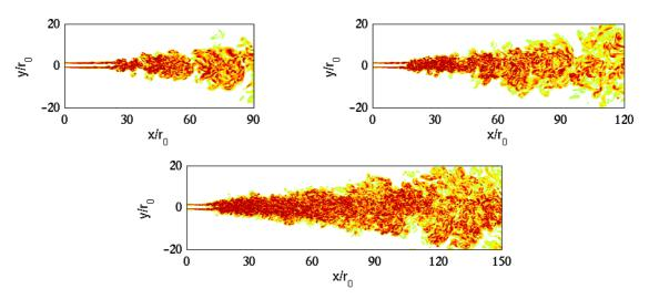
FIG. 1 – Snapshots of vorticity norm normalized by the jet diameter and the centerline mean axial velocity,  $|\omega|D/u_c$ , in the plane z = 0, for : jetRe1800 (top left), jetRe3600 (top right) and jetRe11000 (bottom). The color scale ranges for levels from 0.4 to 2.
