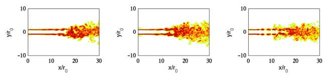
FIG. 2 – Snapshots of vorticity norm normalized by the jet diameter and inflow velocity,  $|\omega|D/u_j$ , in the plane z = 0, for : jetRe3600, jetRe3600thin and jetRe3600mode, from left to right. The color scale ranges for levels from 0.6 to 3.
