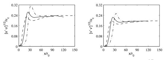
FIG. 5 – Variations along the jet centerline of axial and radial turbulence intensities  $[u'u']^{1/2}/u_c$  (left) and  $[v'v']^{1/2}/u_c$  (right), for : - - - jetRe1800, \_\_\_\_\_\_ jetRe3600, and - - - jetRe11000.
