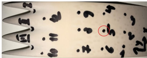
Figure VI.44: Locations of the roughness measurements (black dots).
