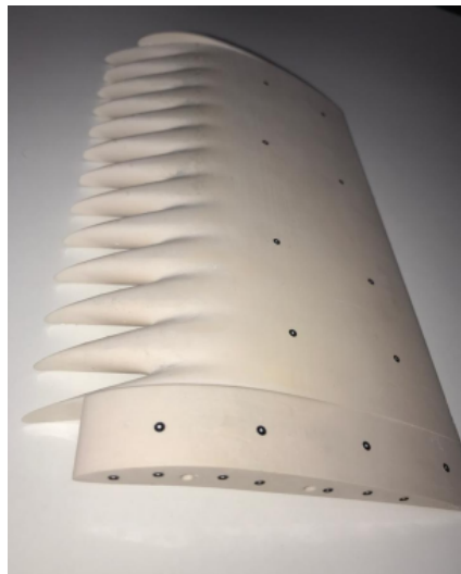
Figure IV.17: 3D serrated vane after support material removal and post-processing.
