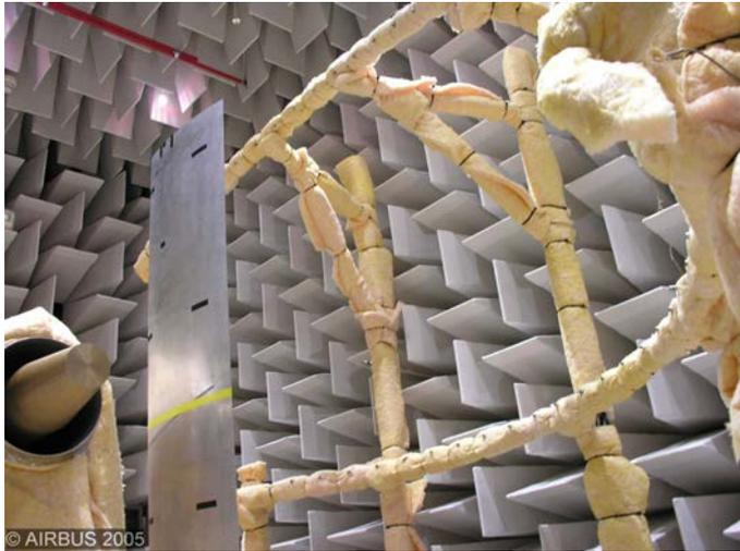
**Figure 5. Exhaust noise shielding experimental set-up in the Airbus anechoic chamber showing the noise simulator, the wing mock-up and the microphones in the flyover and sideline arcs.**
