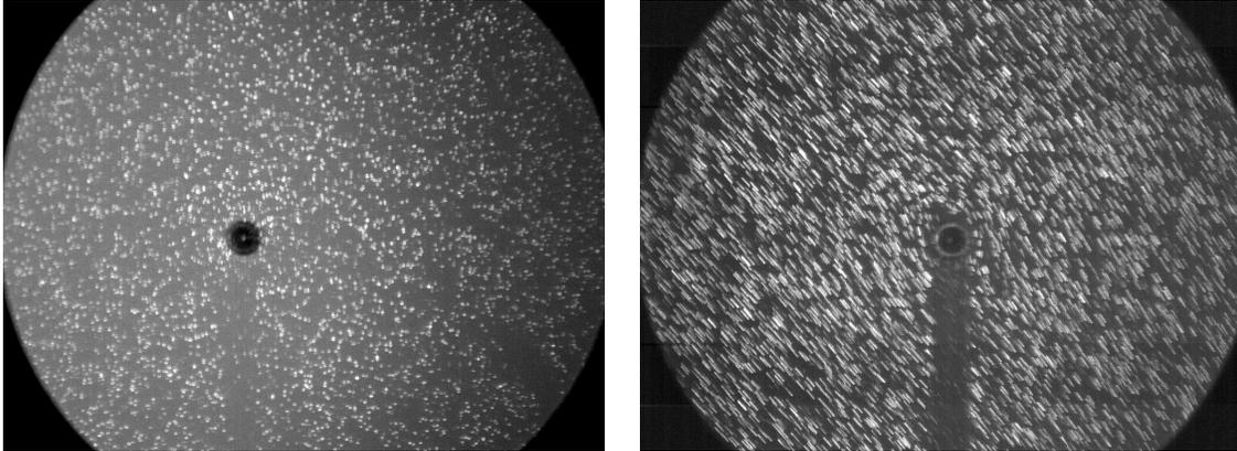
**Figure 2: Fluorescent tracer particles around two bubbles oscillating in a purely spherical mode. Both images correspond to a superposition of 100 snapshots covering 0.25 s. Left: No motion of the tracer particles can be observed. Right: A parasite mean flow can be observed in the whole image. However, this flow is not linked to the bubble motion.**
