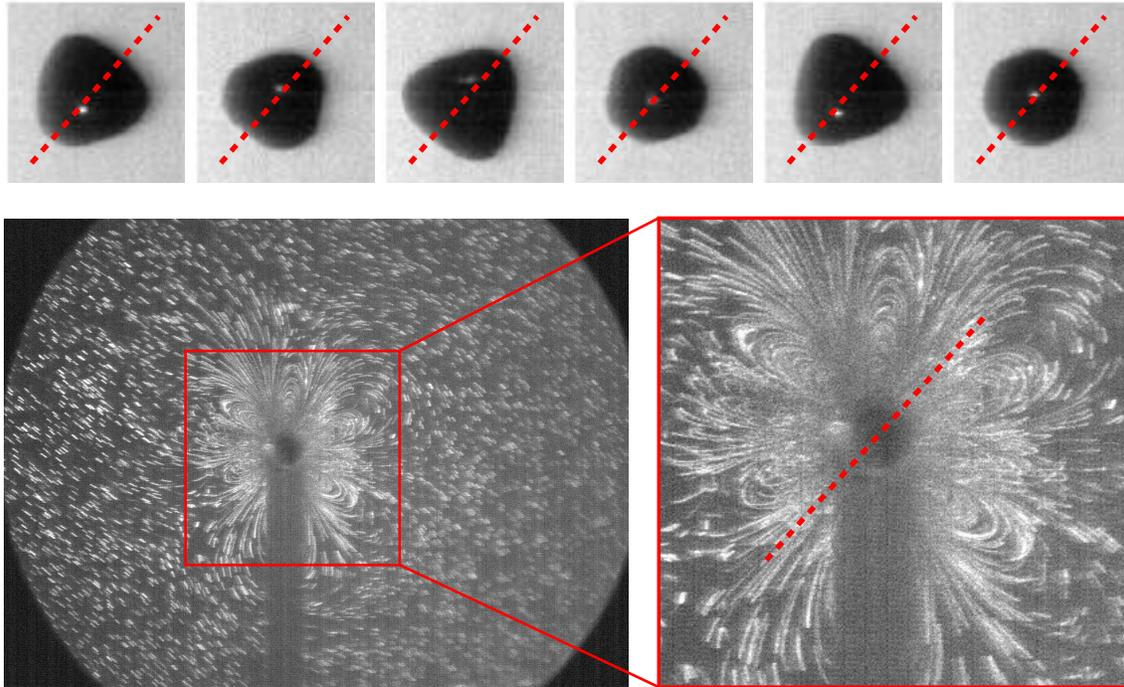
**Figure 3:** Above: Bubble dynamics of bubble oscillating in a mode 3, represented by consecutive snapshots over two acoustic periods (0.064 ms). The axis of symmetry is indicated by the dashed red line. Below: Streaming pattern induced by this bubble. The image corresponds to a superposition of 100 snapshots covering 0.25 s. The width and height of the red box are 0.7 mm.
