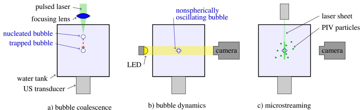
**Figure 1: Experimental setup using the following steps: a) triggering of surface modes by bubble coalescence, b) recording of the bubble dynamics, c) recording of the microstreaming.**
