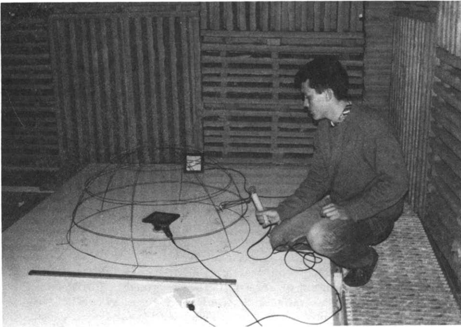
Fig. 5. Acoustic power measurement by intensimetry.
